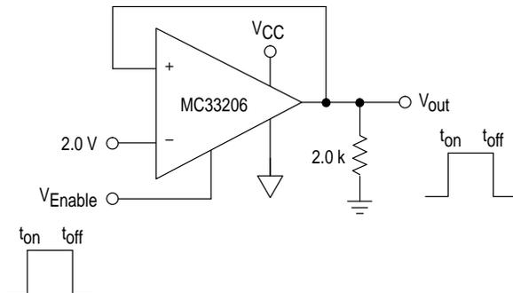
**Figure 28.  $t_{on}$  Response**
