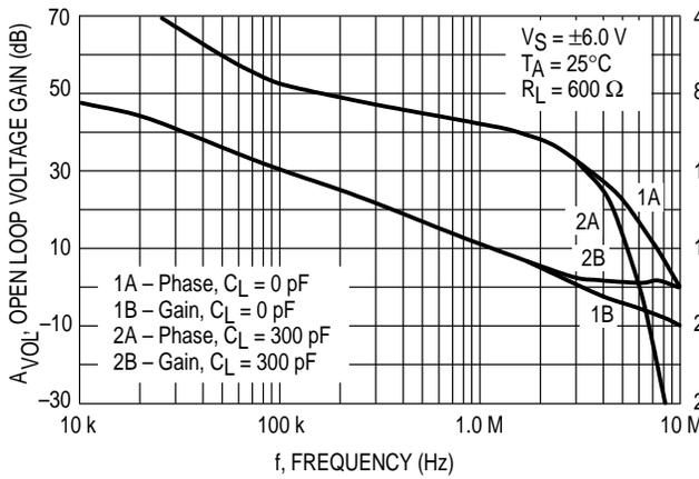
Figure 19. Voltage Gain and Phase versus Frequency
