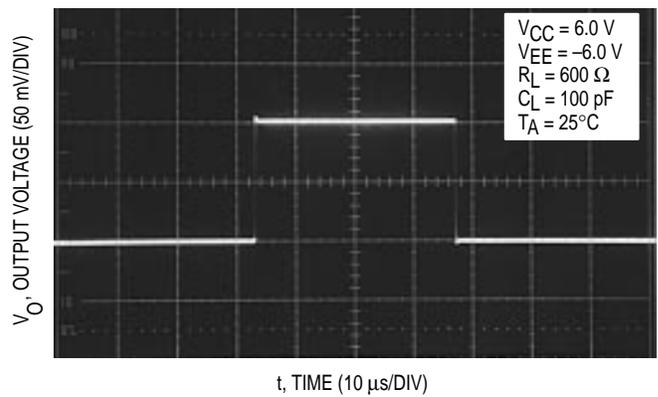
Figure 34. Large Signal Transient Response
