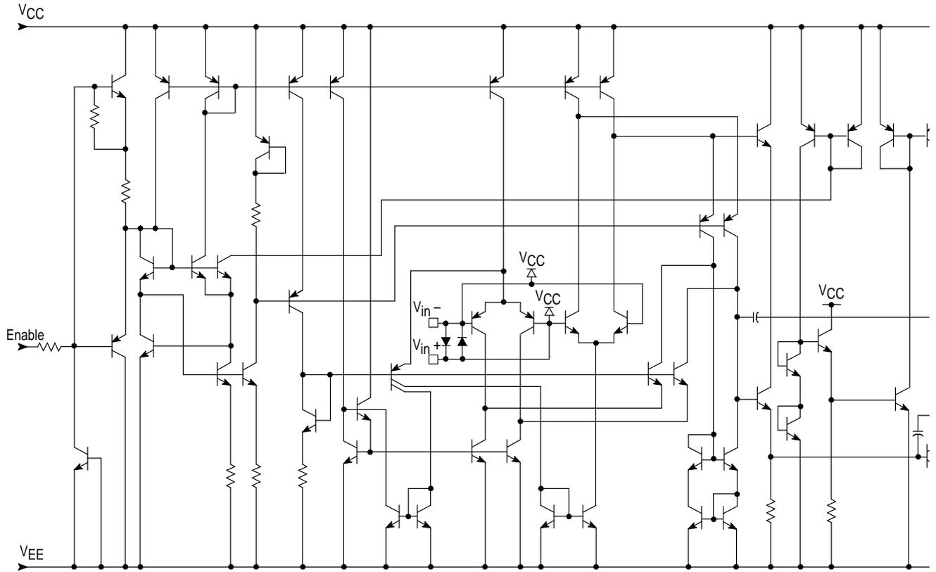
This device contains 96 active transistors (each amplifier).
