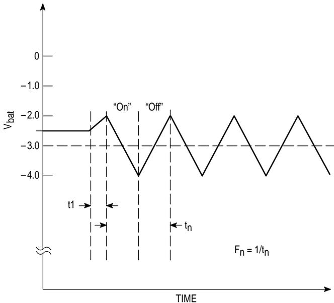
**Figure 2. One Defective Lamp Oscillator Timing Diagram**
