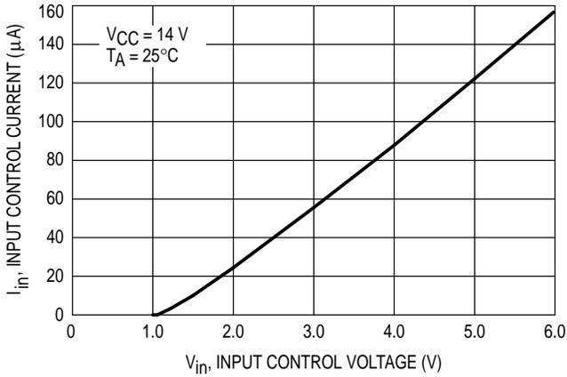
**Figure 5. Input Control Current versus Supply Voltage**
