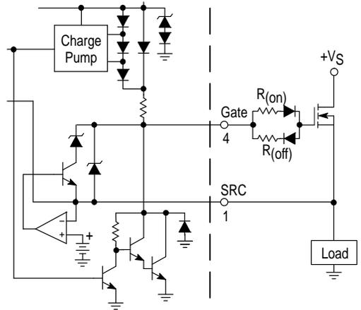
Figure 35. Decreased FET Turn-Off Time with Inductive Flyback Voltage Clamp
