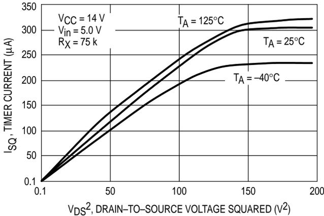
**Figure 9. Timer Current versus Drain-to-Source Voltage Squared**
