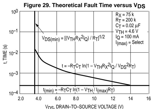
When driving incandescent lamp loads, the minimum timer time-out (time required for the  $V_T$  voltage to reach  $V_{TH}$  threshold of the upper comparator) should be set long enough so as to *not* allow the in-rush current of incandescent lamp to cause a false trigger, yet short enough to afford the TMOS device survival protection against direct shorts under worst case supply and temperature conditions.
