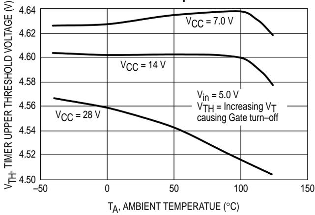
Figure 11. Timer Upper Threshold Voltage versus Supply Voltage
