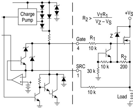
Figure 36. Overvoltage Protection of FET
