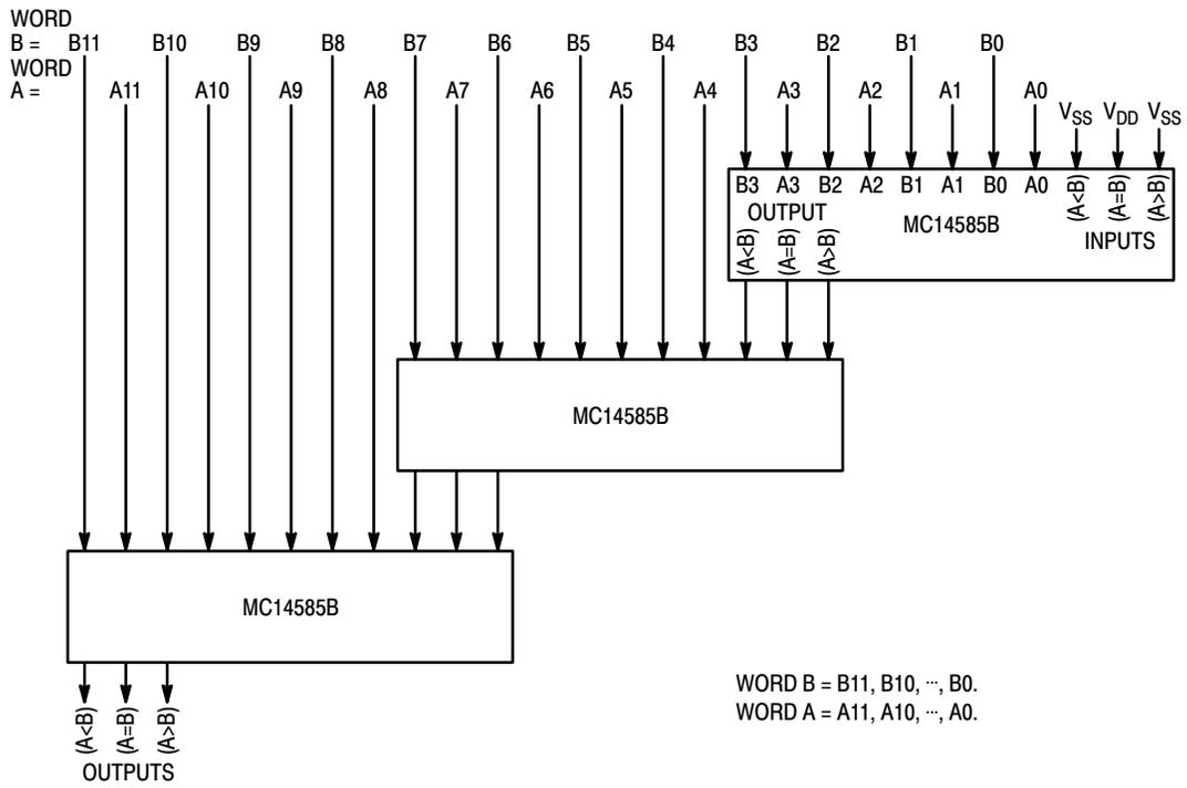
Figure 3. Cascading Comparators
