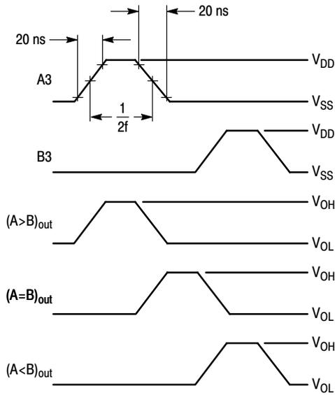
Inputs (A>B) and (A=B) high, and inputs B2, A2, B1, A1, B0, A0 and (A<B) low.
