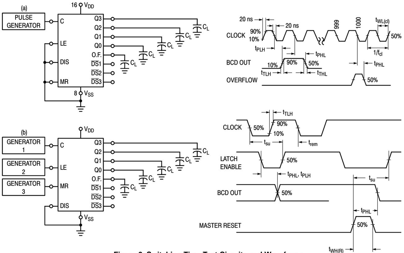
Figure 2. Switching Time Test Circuits and Waveforms
