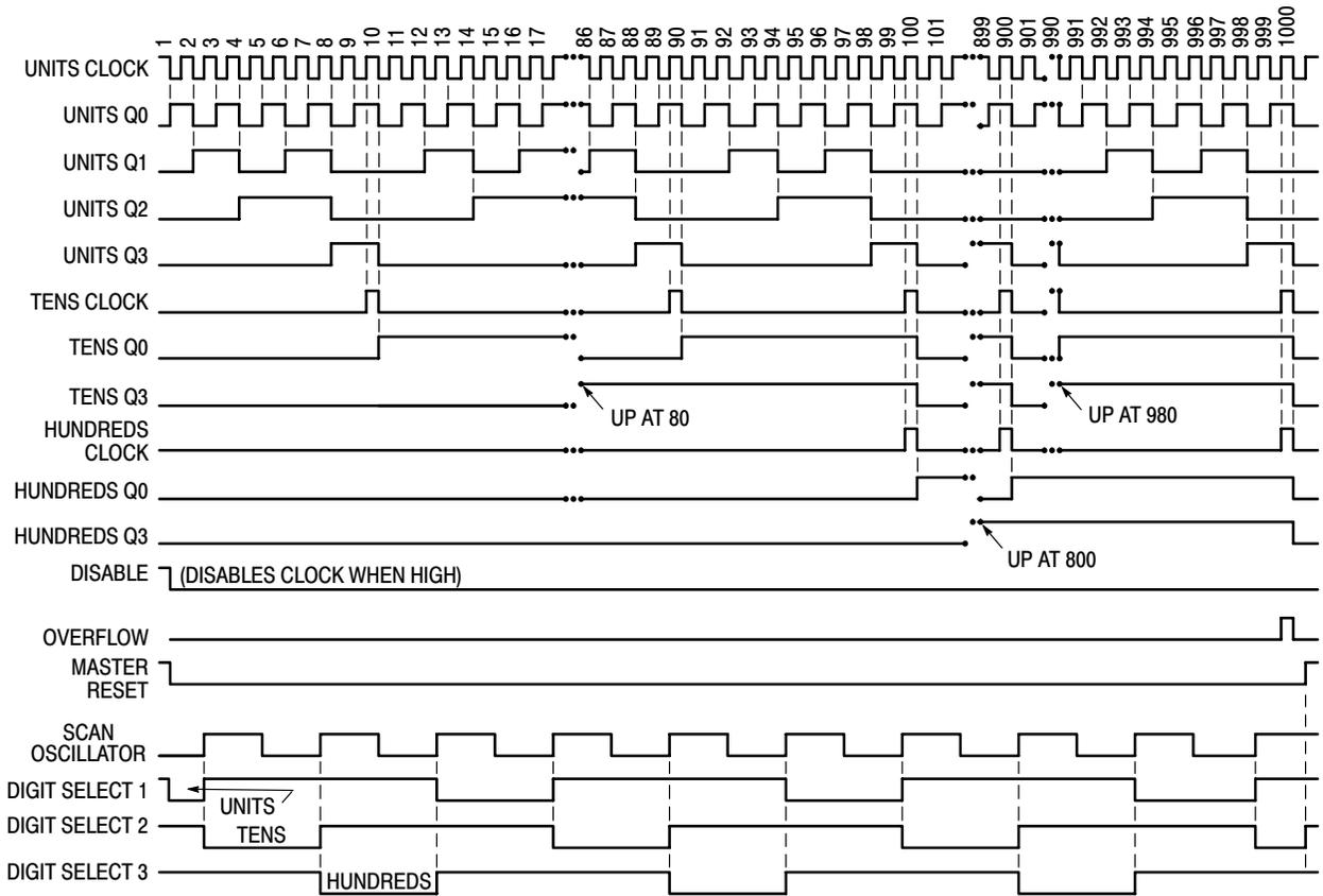
Figure 1. 3-Digit Counter Timing Diagram (Reference Figure 3)
