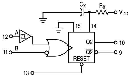
R<sub>X</sub> AND C<sub>X</sub> ARE EXTERNAL COMPONENTS.
