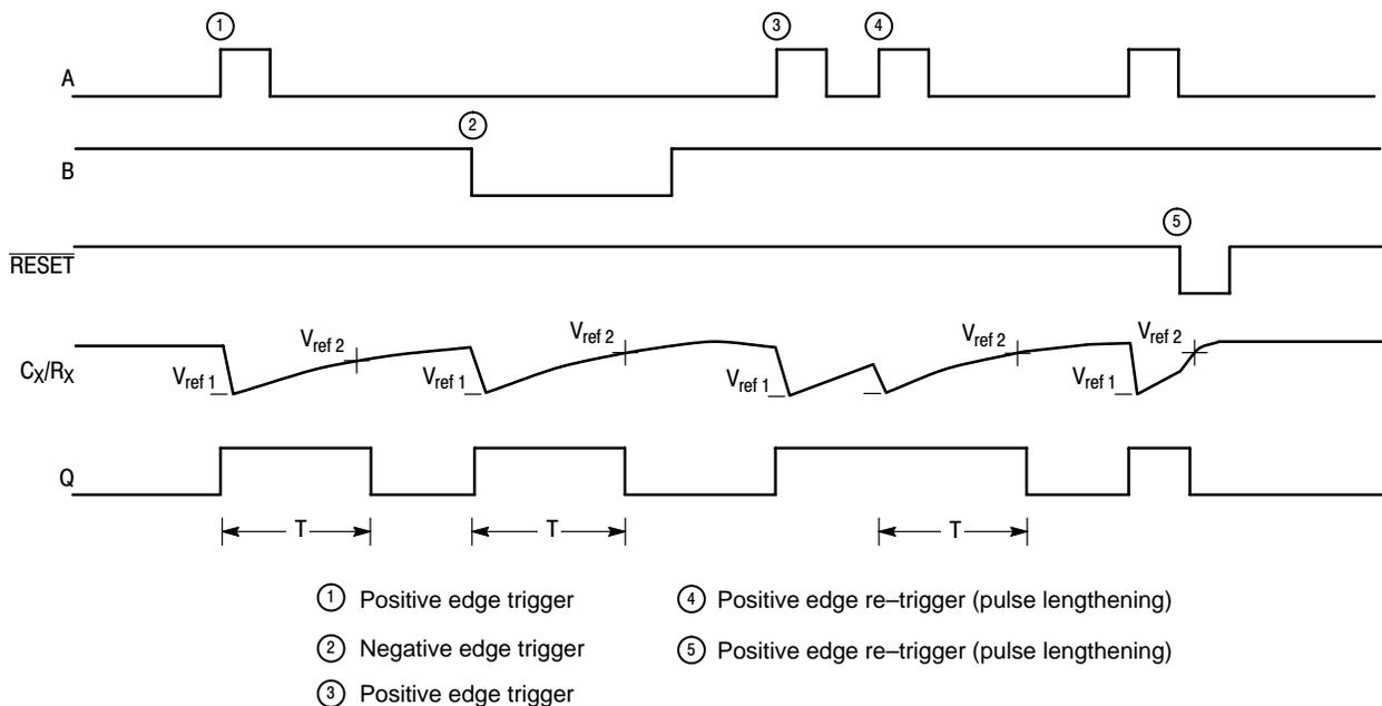
Figure 10. Timing Operation
