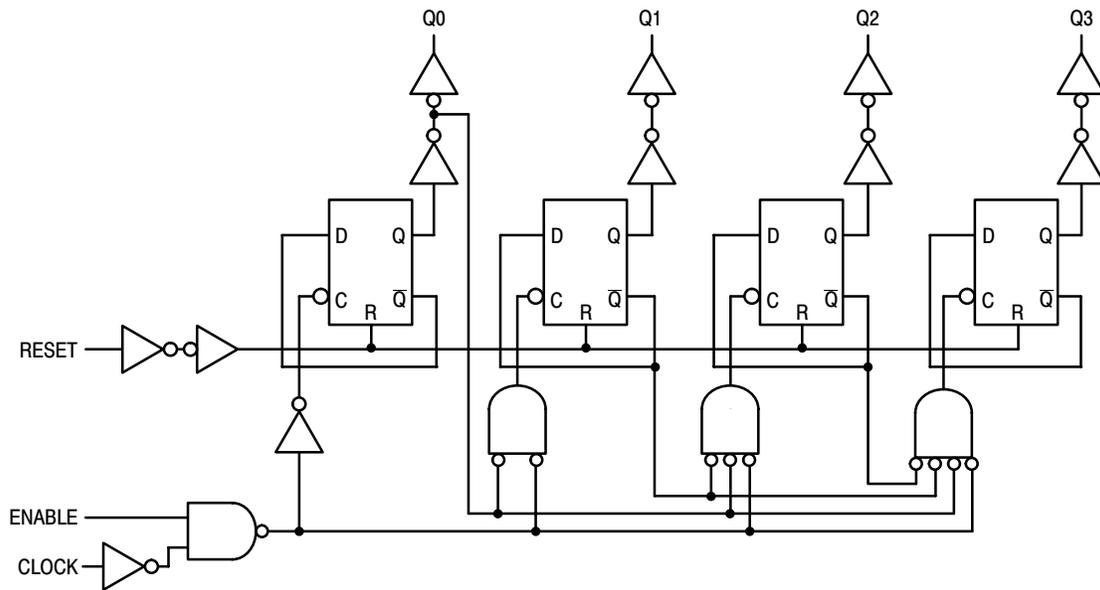
Figure 5. Binary Counter (MC14520B) Logic Diagram
