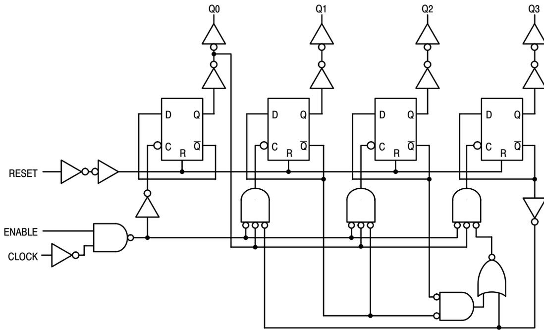
Figure 4. Decade Counter (MC14518B) Logic Diagram
