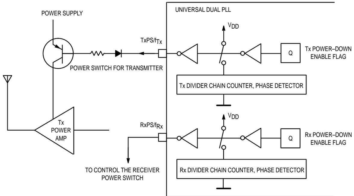
**Figure 17. TxPS/f<sub>Tx</sub> and RxPS/f<sub>Rx</sub> Outputs to Control Power Switches of the Transmitter and the Receiver**
