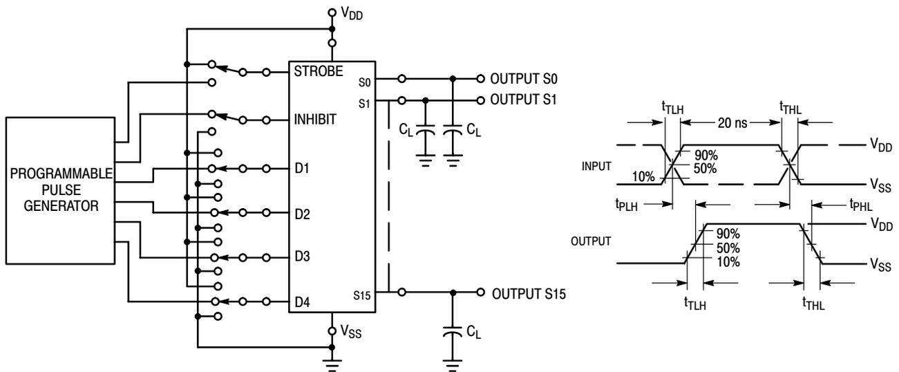
Figure 3. Switching Time Test Circuit and Waveforms
