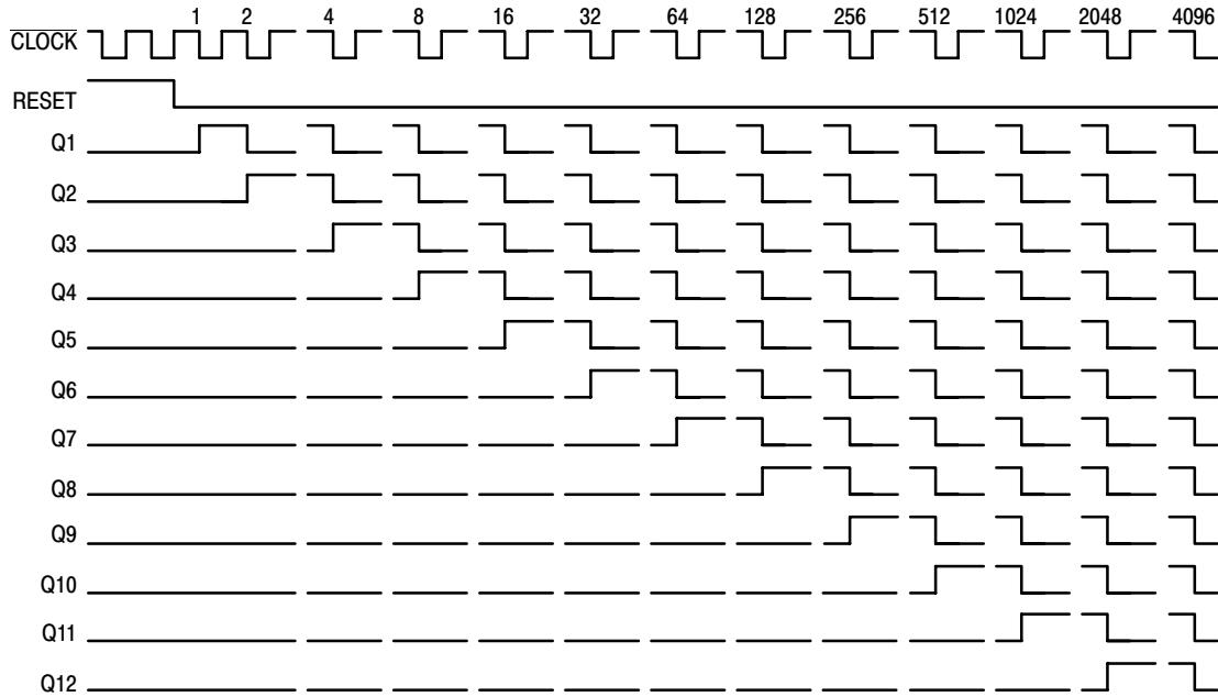
**Figure 3. Timing Diagram**
