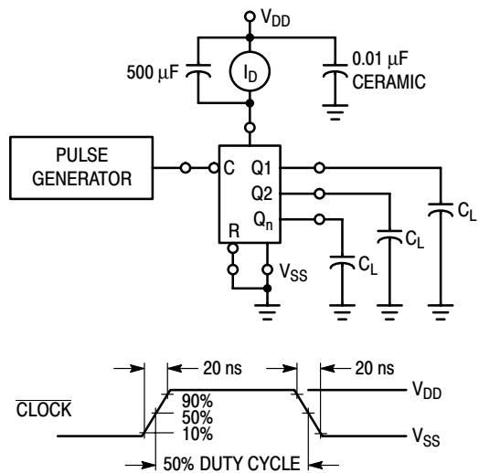
**Figure 1. Power Dissipation Test Circuit and Waveform**
