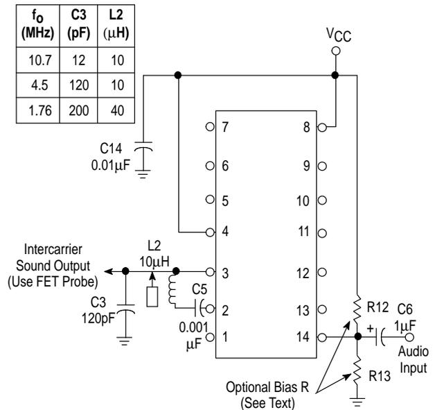
**Figure 12. Modulator Sensitivity**
