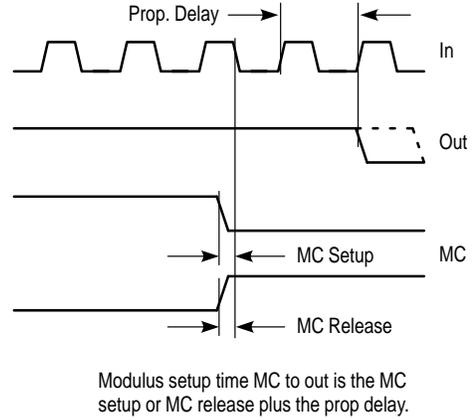
Figure 3. Typical Output Waveforms
