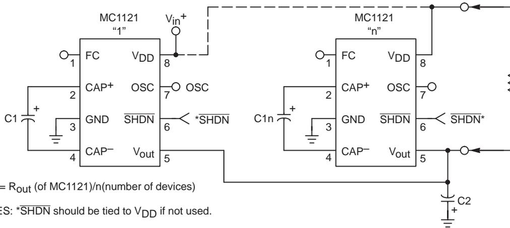
$$R_{out} = R_{out} \text{ (of MC1121)}/n(\text{number of devices})$$
