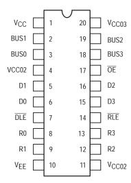
Pin assignment is for Dual–in–Line Package.
