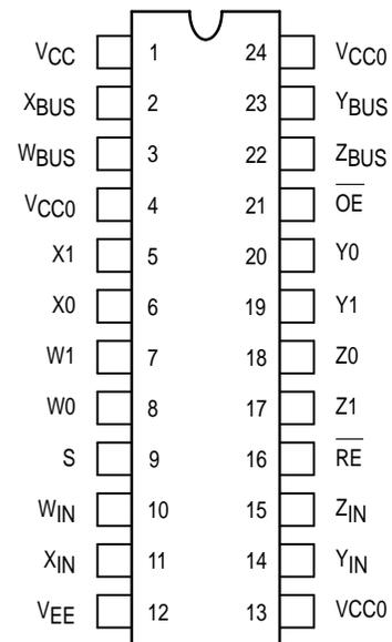
Pin assignment is for Dual-in-Line Package. For PLCC pin assignment, see the Pin Conversion Tables on page 6-11 of the Motorola MECL Data Book (DL122/D).
