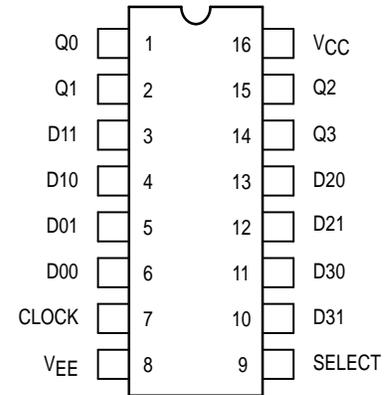
Pin assignment is for Dual-in-Line Package. For PLCC pin assignment, see the Pin Conversion Tables on page 6-11 of the Motorola MECL Data Book (DL122/D).
