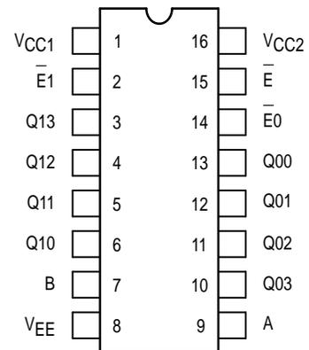
Pin assignment is for Dual-in-Line Package. For PLCC pin assignment, see the Pin Conversion Tables on page 6-36 of the Motorola MECL Data Book (DL122/D).
