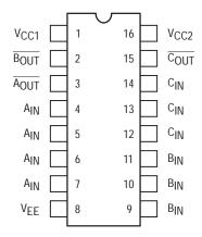
Pin assignment is for Dual-in-Line Package. For PLCC pin assignment, see the Pin Conversion Tables on page 18 of the ON Semiconductor MECL Data Book (DL122/D).
