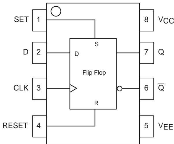
Figure 1. 8-Lead Pinout (Top View) and Logic Diagram
