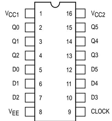
Pin assignment is for Dual-in-Line Package. For PLCC pin assignment, see the Pin Conversion Tables on page 6-11 of the Motorola MECL Data Book (DL122/D).
