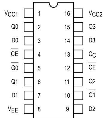
Pin assignment is for Dual-in-Line Package.
