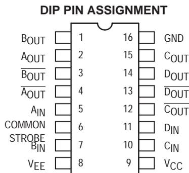
Pin assignment is for Dual-in-Line Package.
