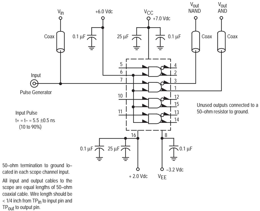
NOTE: All power supply and logic levels are shown shifted 2 volts positive.
