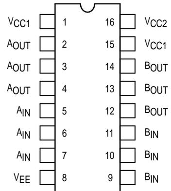
Pin assignment is for Dual-in-Line Package.
