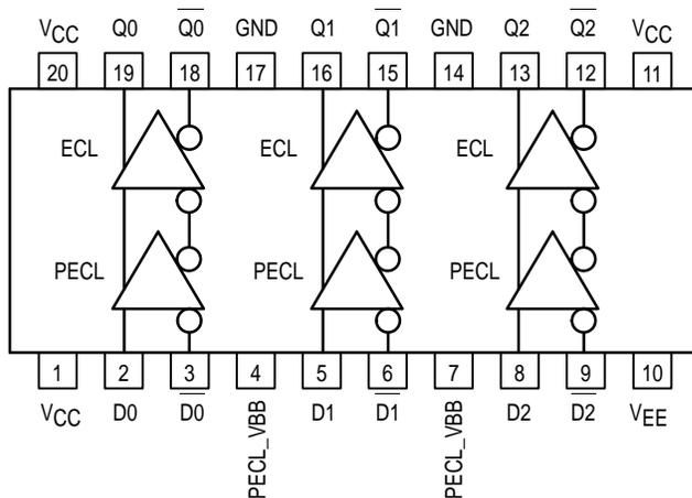
**Figure 1. 20-Lead Pinout (Top View) and Logic Diagram**
