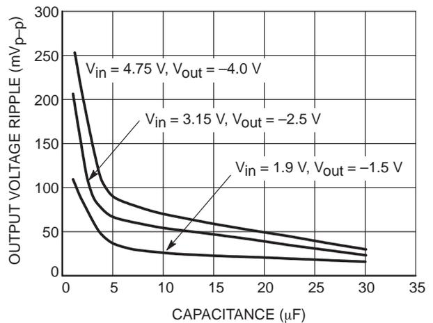
Figure 13. Output Voltage Ripple versus Capacitance (MAX829)
