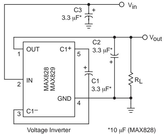
**Figure 3. Test Circuit**
