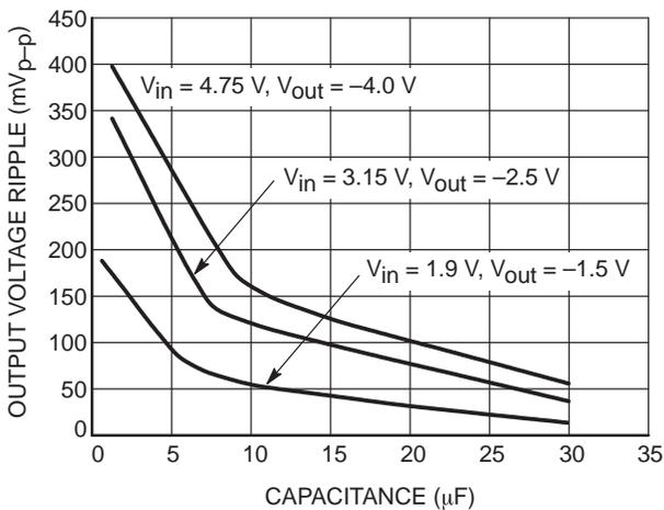
Figure 12. Output Voltage Ripple versus Capacitance (MAX828)
