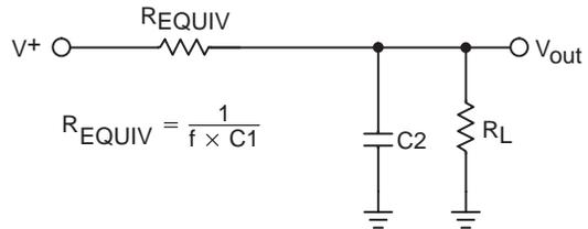
Figure 2b. Equivalent Output Resistance
