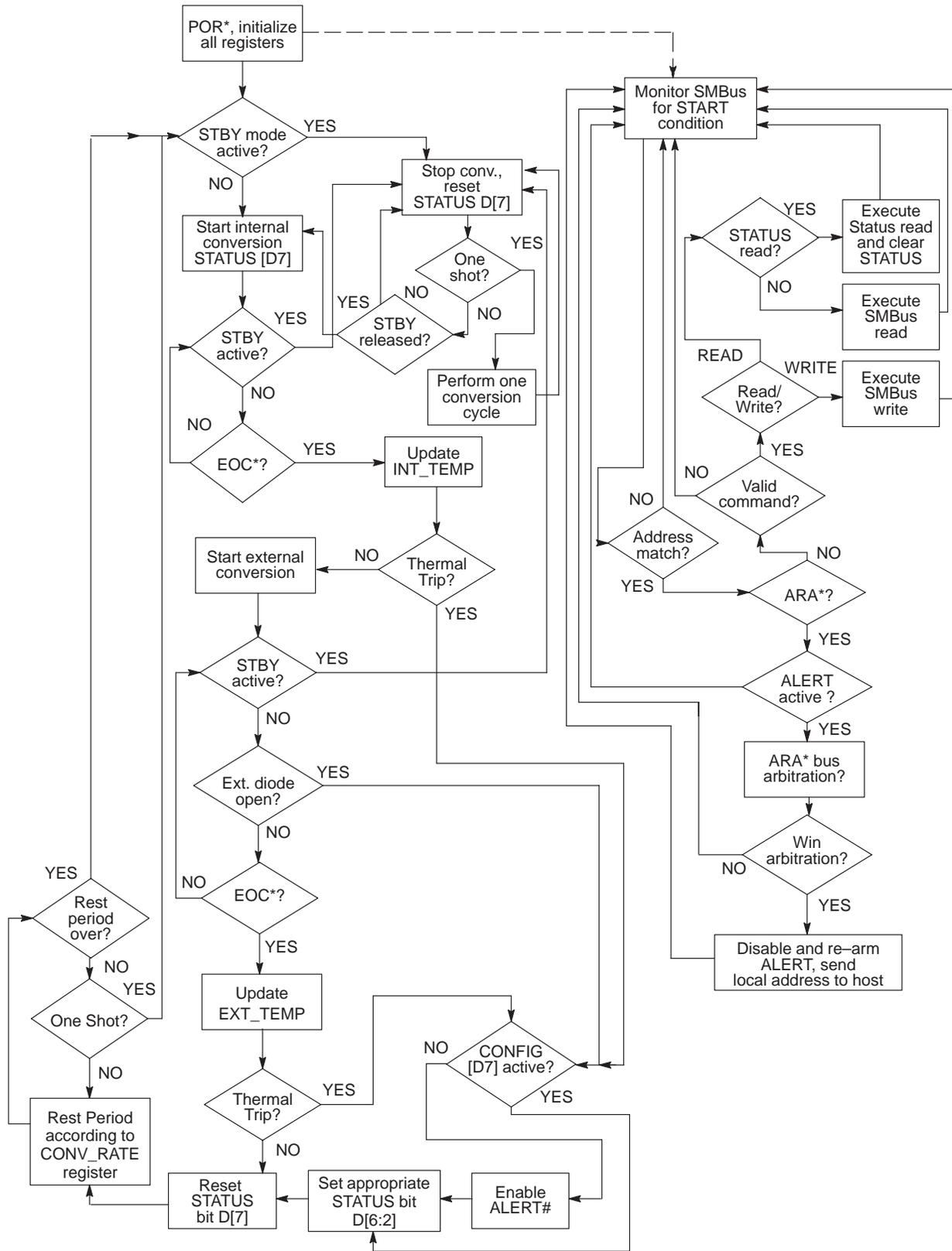
\* POR = Power On Reset; ARA = Alert Response Address; EOC = End Of Conversion
