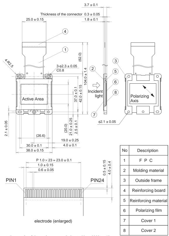
The rotation angle of the active area relative to H and V is  $\pm$  1°.
