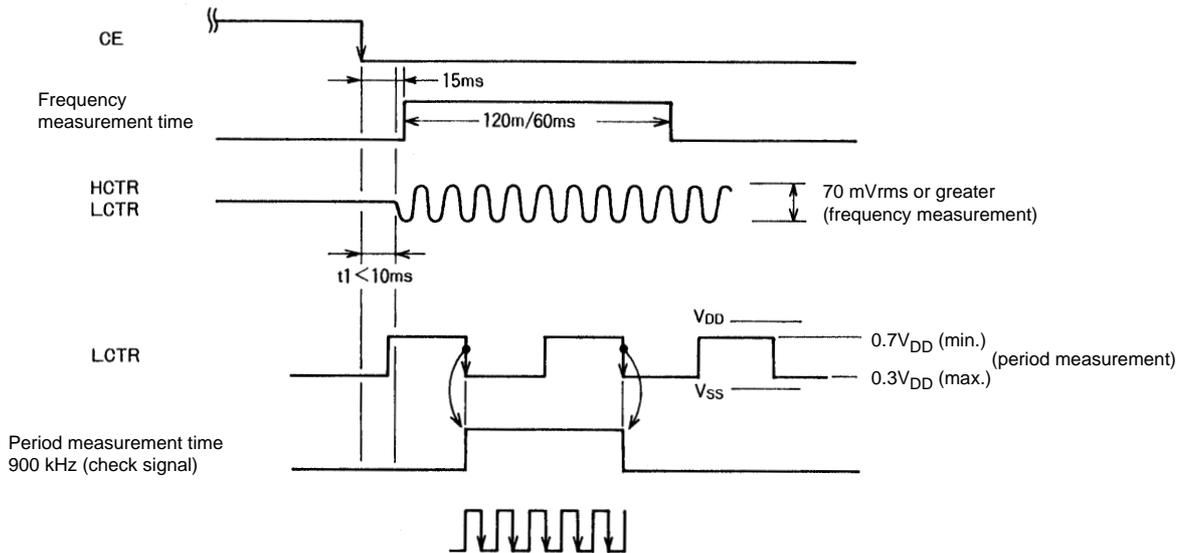
Note that although the DO pin is forced to the high level when the general-purpose counter is started (when CTEN is set to 1), the DO pin automatically goes low when the measurement completes (after either 60 or 120 ms has elapsed or when a signal has been applied for one or two periods). Therefore the DO pin can be used to check for measurement completion.
