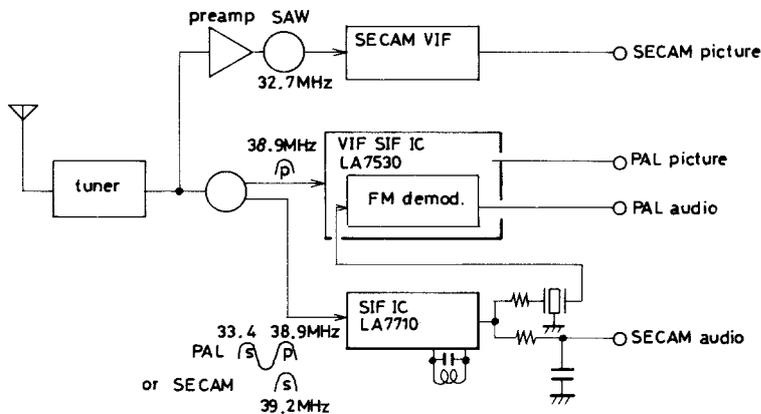
(Note) \*1 When selecting the PAL/SECAM, the LLD tuning point of the LA7710 must be changed over (38.9MHz → 39.2MHz).
