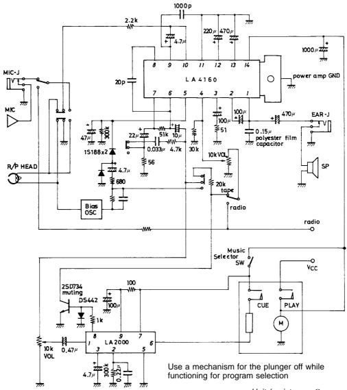
Unit (resistance:  $\Omega$ , capacitance: F)
