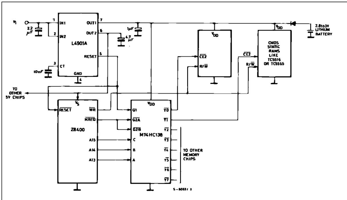
Another interesting application of the L4901A is in  $\mu$ P system with shadow memories (see Figure 6). When the input voltage goes below  $V_{IT}$ , the reset output enables the execution of a routine that saves the machine's state in the shadow RAM (xicor x 2201 for example).
