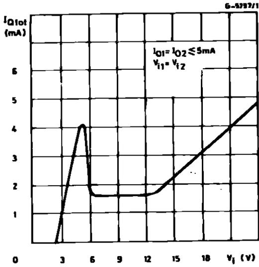
**Figure 10 :** Regulator 1 Output Current and Short Circuit Current versus Input Voltage
