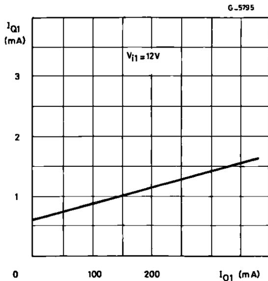
Figure 8 : Quiescent Current (reg.1) versus Input Voltage
