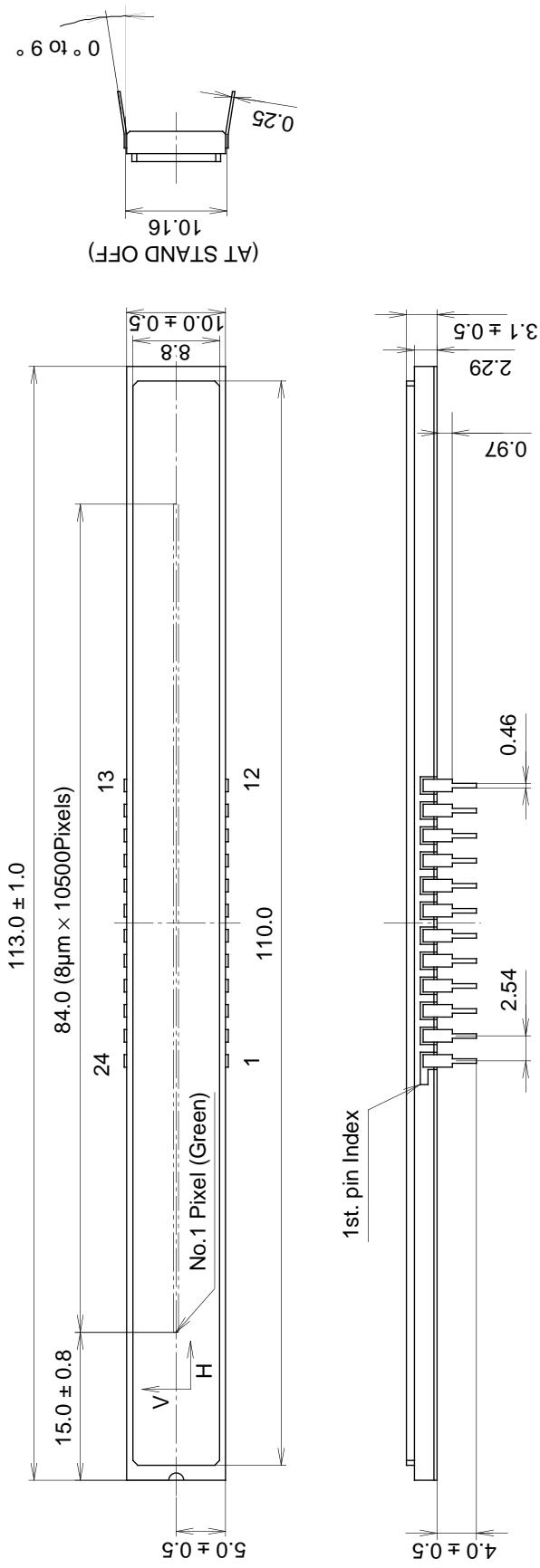
1. The height from the bottom to the sensor surface is 1.42mm ±0.4.
