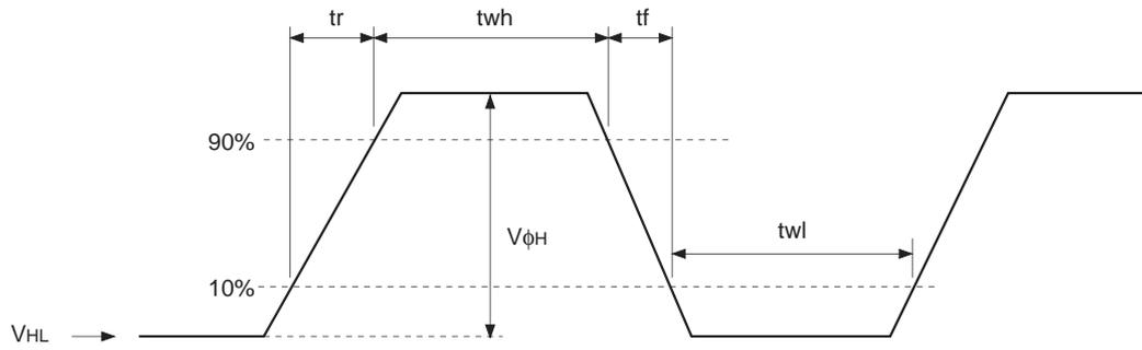
**(4) Reset gate clock waveform**
