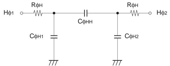
**Horizontal transfer clock equivalent circuit**
