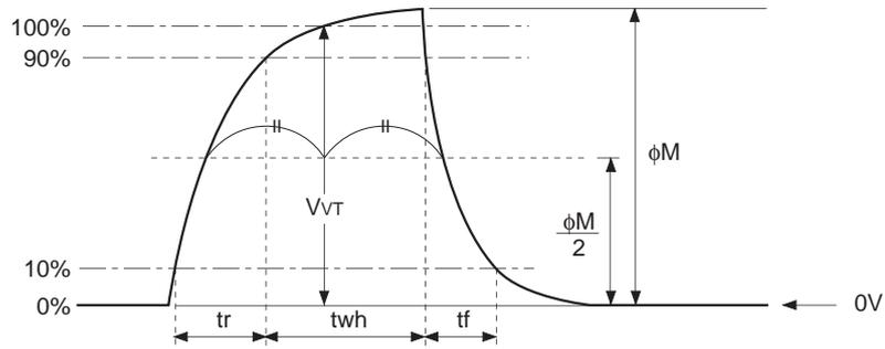
(2) Vertical transfer clock waveform
