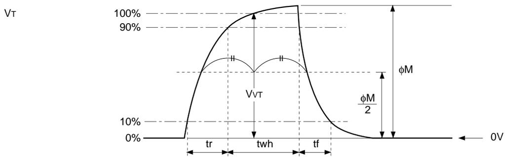
(2) Vertical transfer clock waveform
