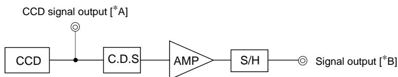
**Note)** Adjust the amplifier gain so that the gain between [\*A] and [\*B] equals 1.
