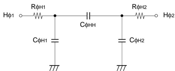
**Horizontal transfer clock equivalent circuit**
