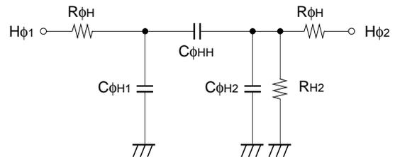
**Horizontal transfer clock equivalent circuit**
