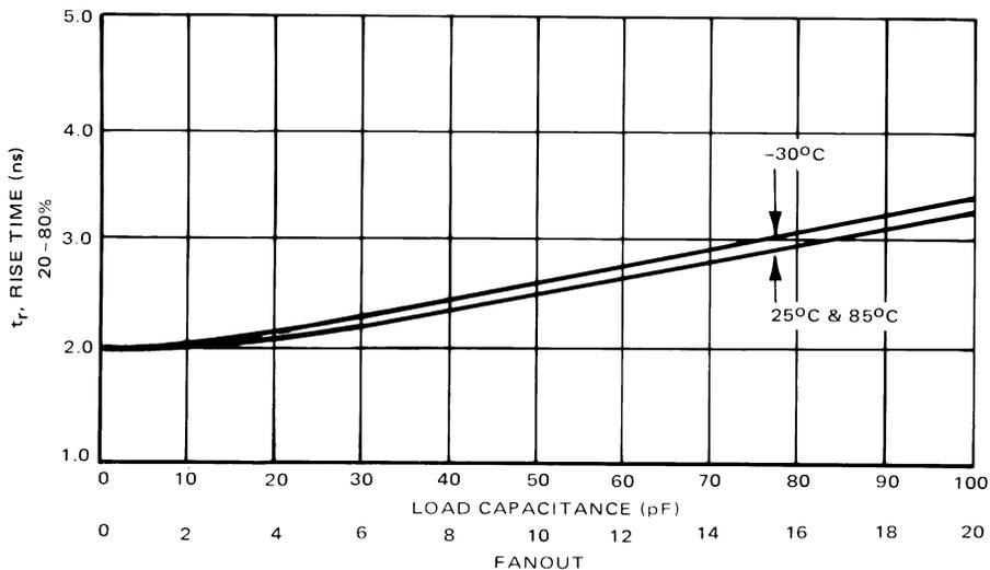
2-2: Rise Time versus Loading and Temperature (MECL 10K)
