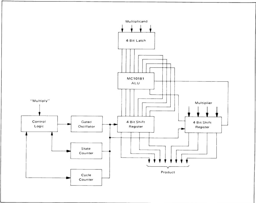
FIGURE 38 — 4 x 4 Bit MECL 10K Multiplier
