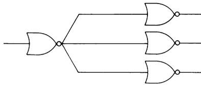
This technique should be used for shift register clocks, counter resets, and other high fanout applications. Of course, for synchronous clock lines, clock skew delays should be matched. Series damping may also be used with parallel signal paths.
