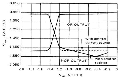
FIGURE 3 — Typical MECL 10K Transfer Characteristics
