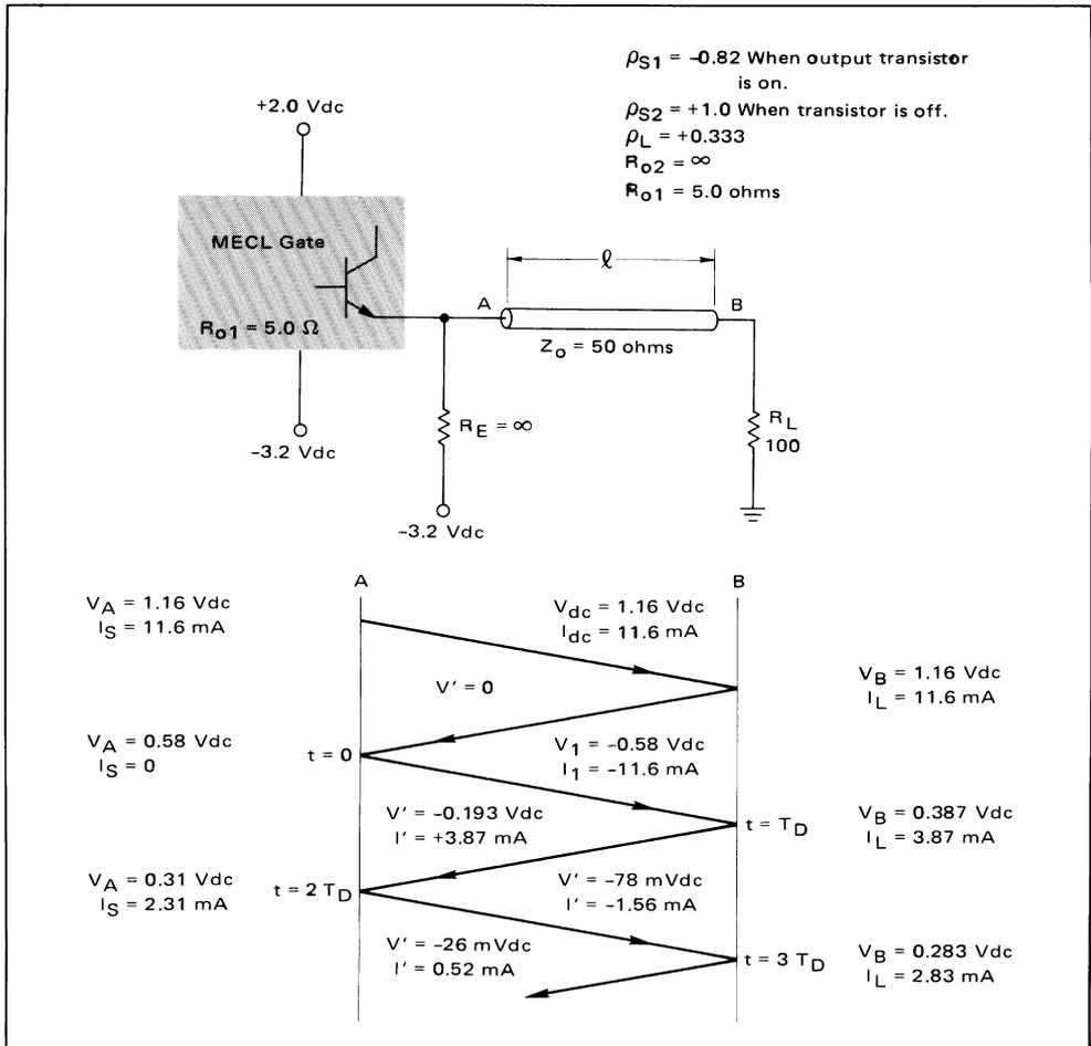
*Voltage Waveforms as a Function of Time*
