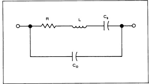
FIGURE 2 — Equivalent Circuit of a Quartz Crystal
