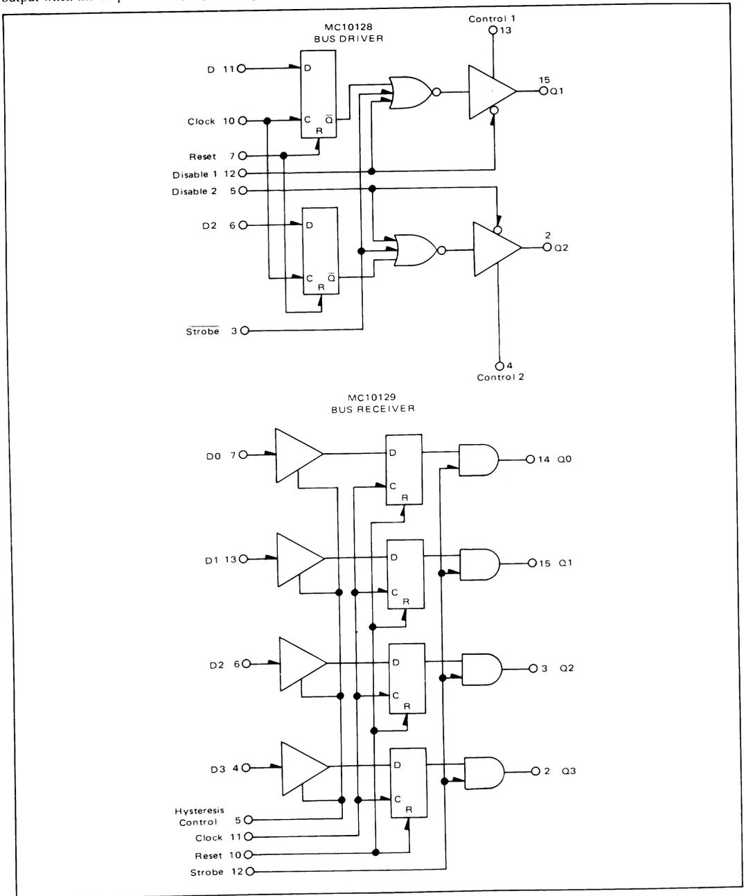
FIGURE 4 – MECL to IBM or TTL Interface Circuits
