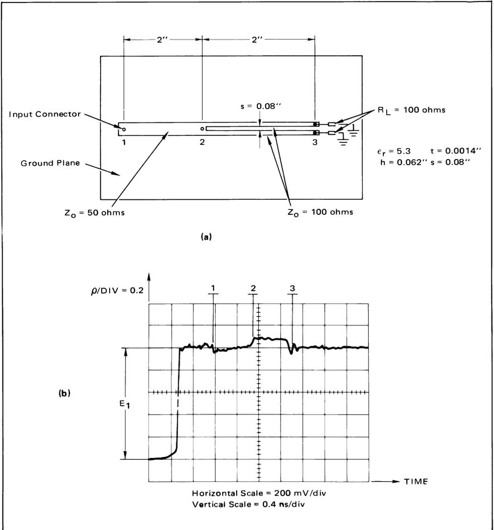
Even mode or odd mode characteristic impedance ( $Z_{oe}$  or  $Z_{oo}$ ) can be considered to exist in a circuit with crosstalk. One,  $Z_{oe}$ , is due to the strips being at the same potential and carrying equal currents in the same direction. The other,  $Z_{oo}$ , is due to the strips being at equal but opposite potentials and carrying equal currents in opposite directions. The backward crosstalk voltage,  $V_B$ , on a passive line is given in Reference 10 as:
