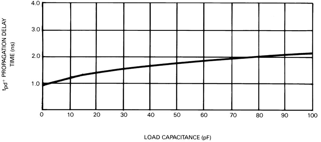
2-8: Propagation Delay,  $t_{pd-}$ , versus Loading (MECL 10KH)
