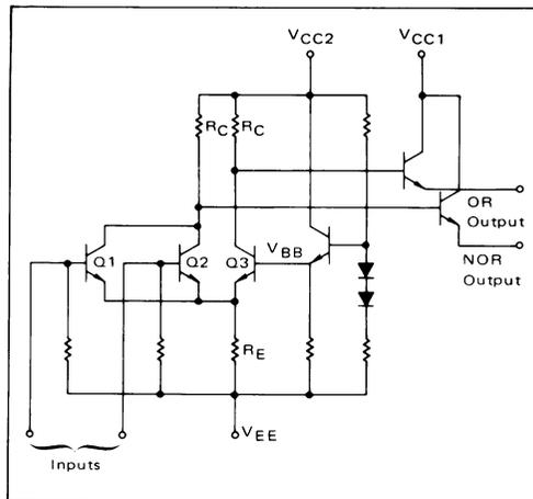
FIGURE 8 - MECL GATE SCHEMATIC
