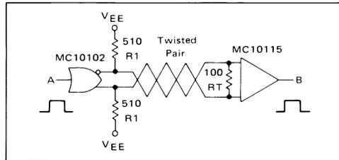
FIGURE 25 – Twisted Pair Line Driver and Receiver
