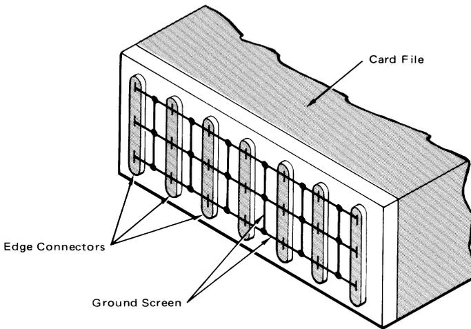
used as a ground, providing connection points for the ground grid. This interconnection of ground points forms a grid network of approximately 1 inch squares over which the signal lines are wired. A characteristic impedance for a wire over ground screen of about 140 ohms can be expected, depending upon the exact routing and distance from the ground screen. The capacitance of this type line will be about 1 to 2 pF per inch, and series inductance will be about 20 nH per inch.
