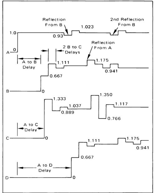
FIGURE 10 — Waveforms of Figure 6 Lattice Diagram
