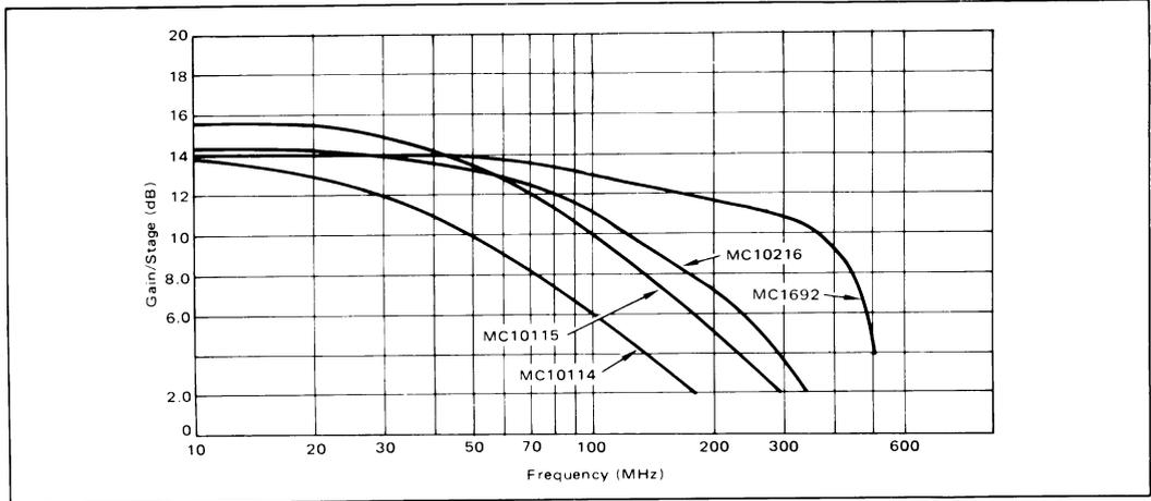
FIGURE 13 – Gain versus Frequency for MECL Line Receivers
