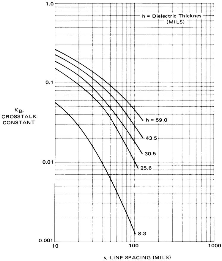
simultaneously, the reflection observed on the TDR is twice as much, or 11%. From Figure 7-15, the actual crosstalk can be seen to be about 8%.
