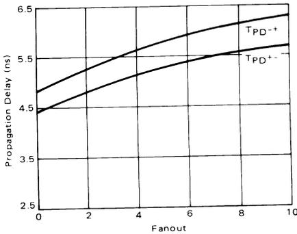
FIGURE 2 — Propagation versus Fanout for the MC10125
