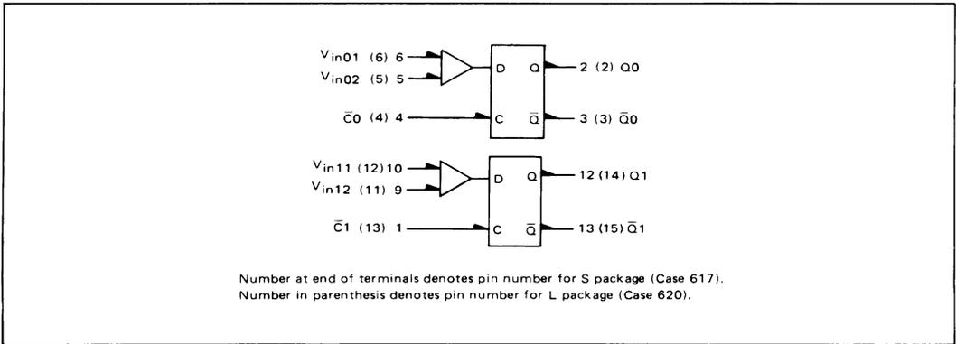
FIGURE 15 – MC1650 Dual A/D Comparator
