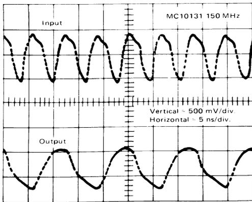
FIGURE 6 – MC10131 Toggle Rate Test
