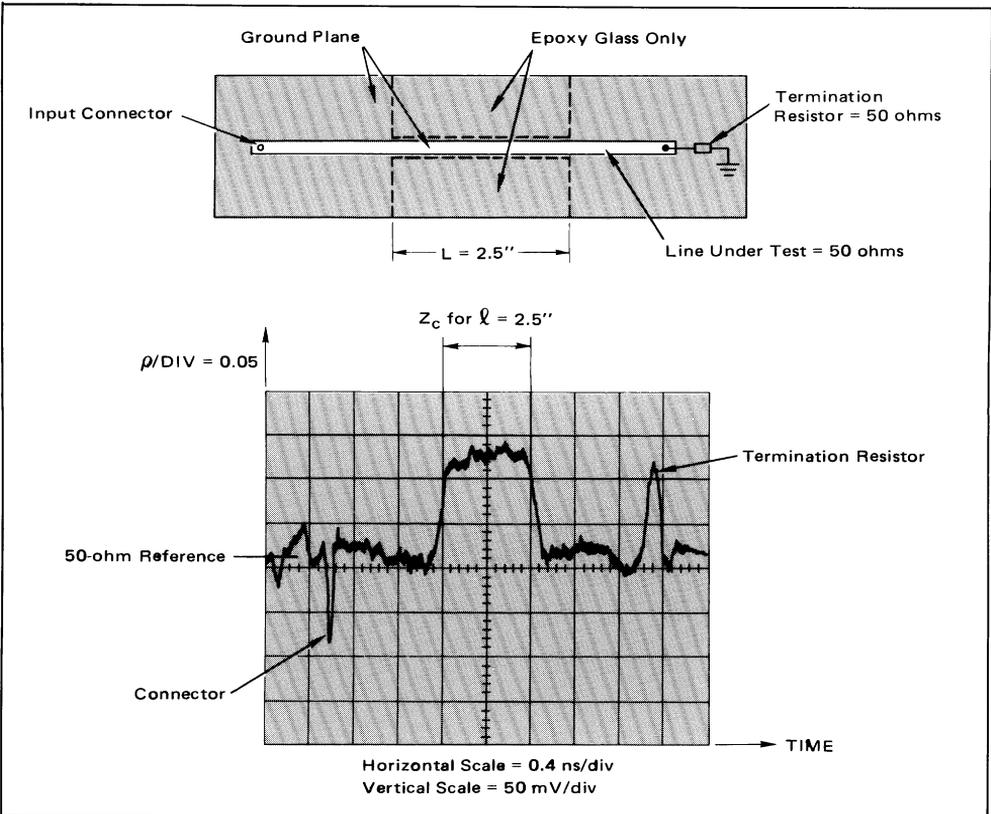
illustrates what happens when the ground plane width under the transmission line abruptly drops to the width of an active line. The TDR waveform shows that a 12% reflection occurs due to this discontinuity in the ground plane.
