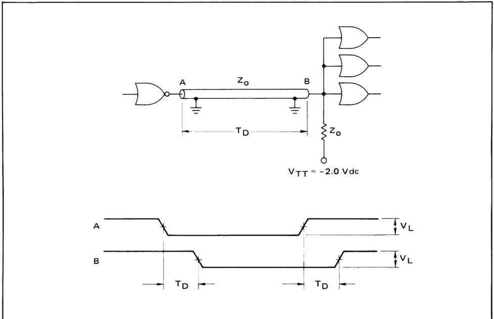
represents the delay of the line. Since a full logic swing is available all along the line, parallel termination permits distributed loading to be placed anywhere along the line.
