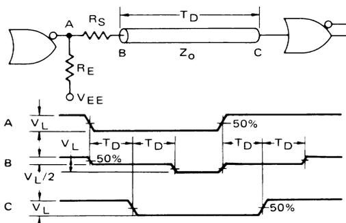
The impedance looking back toward the driving gate at point B should be equal to the characteristic impedance of the transmission line. The dc output impedance is 5 ohms for a MECL III gate and 7 ohms for a MECL 10K/10KH gate. AC output impedance is only slightly higher than the dc impedance values. Therefore, if  $Z_O$  is 75 ohms, then the value of  $R_S$  must be approximately 68 ohms.
