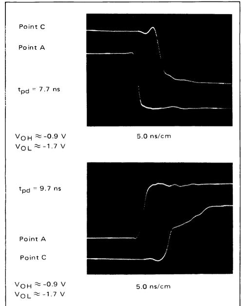
FIGURE 2 – Bus Waveforms With MC10111 Drivers
