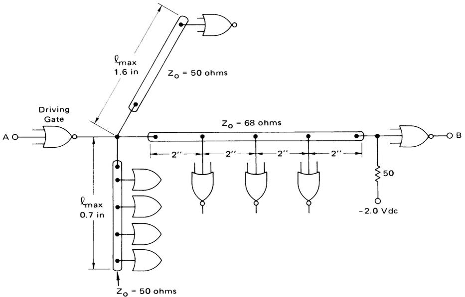
gates on the stub ( $\ell_{\max} = 0.7$  inch) could be lumped at the end of that line, without the need for any other changes.
