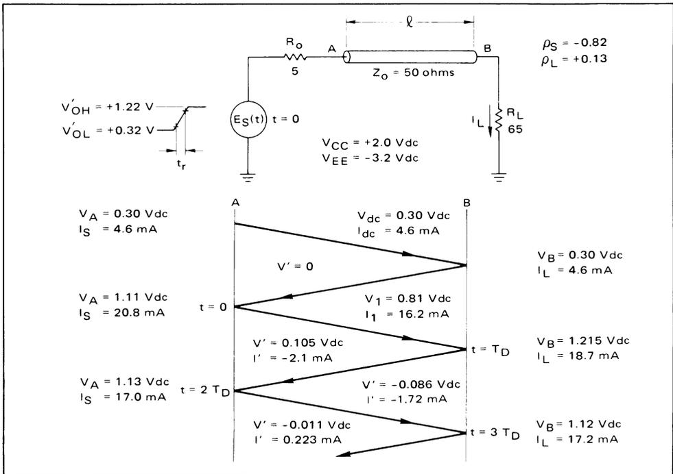
finding  $V(X, t)$  and the use of equation 5. The source impedance of the MECL III gate is 5 ohms, resulting in a reflection coefficient at the source of  $-0.82$  for a line impedance of 50 ohms.
