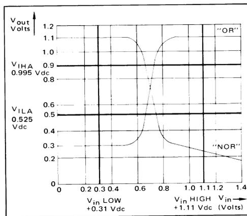
FIGURE 6 — MECL 10K TRANSFER CHARACTERISTICS
