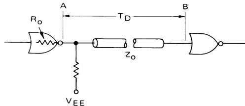
If the lines are sufficiently short, the signal still will be rising at time  $T_D$ , and reflections are part of the rising edge. With longer lines, the rise of the signal will be completed before a time  $T_D$ , and reflections will appear as overshoot and
