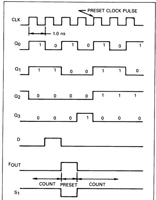
FIGURE 7 – Pulse Diagram for Pulse Gobbling Technique
