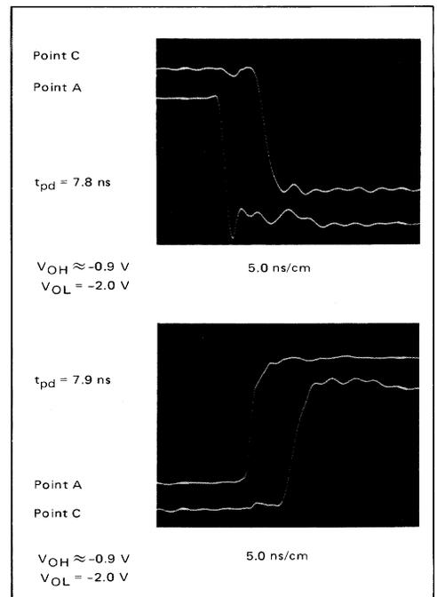
FIGURE 3 — Bus Waveforms With MC10123 Drivers
