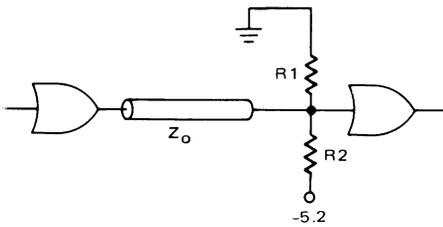
THEVENIN EQUIVALENT RESISTORS FOR TERMINATION
