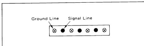
**FIGURE 23 – Cross-Section of a Typical Multiconductor Ribbon Cable**
