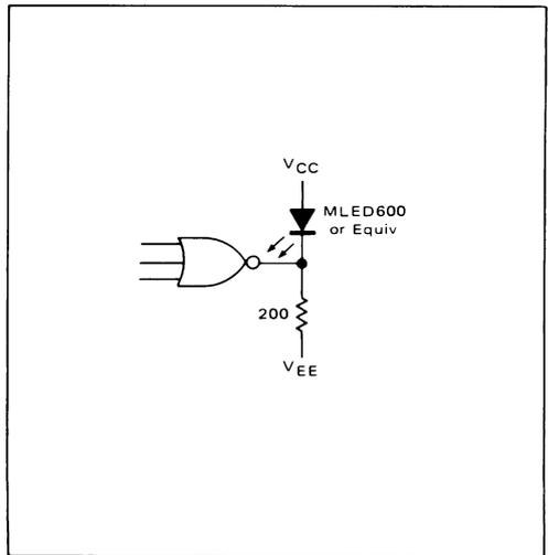
FIGURE 16 – MECL Driving a LED
