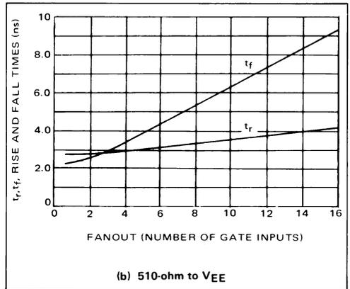
FIGURE 16 — Rise and Fall Time (10 to 90%) versus Fanout
