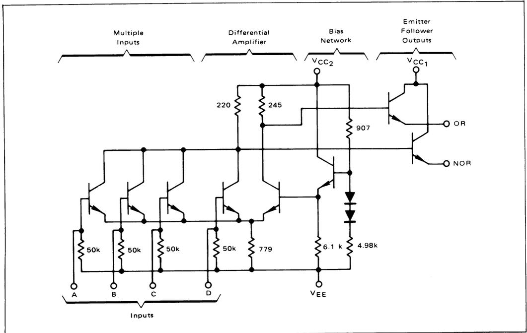
FIGURE 1 — Basic MECL 10K Gate Configuration
