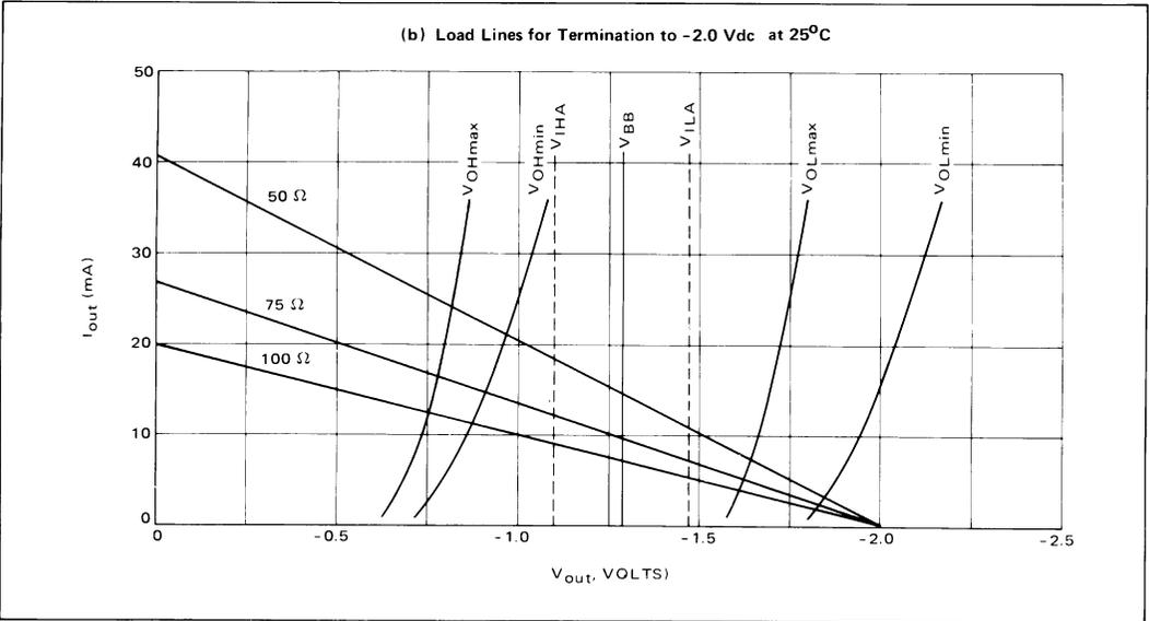
**FIGURE 18 — MECL 10K Operating Characteristics**
