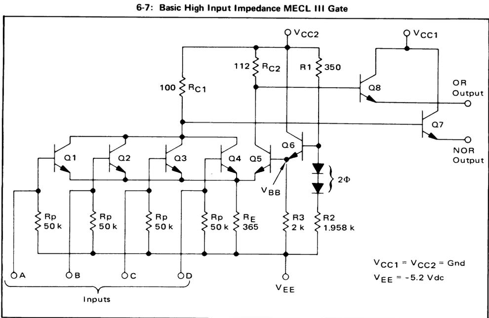
If loop equations are written for the bias supply, the expression obtained for  $V_{BB}$  is:
