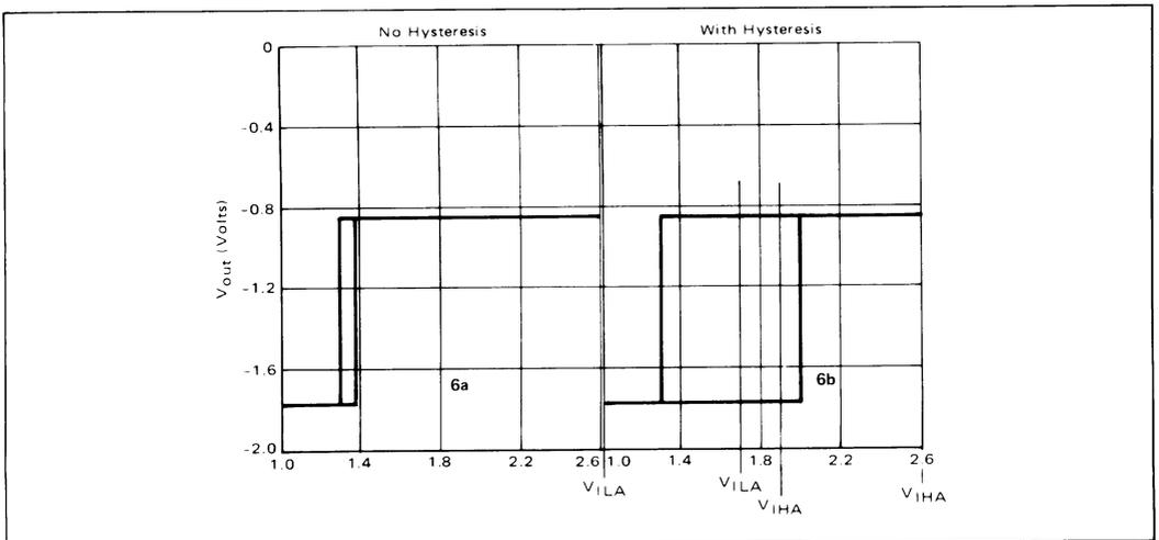
FIGURE 6 - Transfer Characteristics of the MC10129 Bus Receiver
