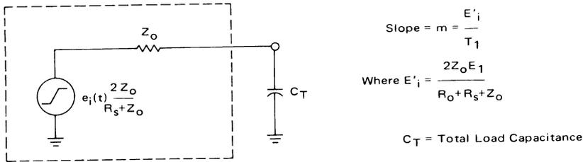
The equations for the output voltage from a series terminated line were derived previously (equations 48 and 49). Since the amplitude has been modified by the factor  $(2Z_o/R_o + R_S + Z_o)$ , a simple substitution will define the output voltage at the load. The output voltage for a series damped line can be written as:
