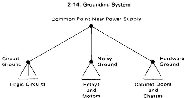
point will eliminate noise on the signal ground (cf Figure 2-14). Heavy ground leads should be used on large systems to minimize any voltage drop along the ground line run.
