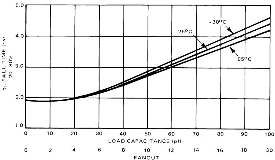
MECL 10K/10KH Parameters versus Loading and Temperature
