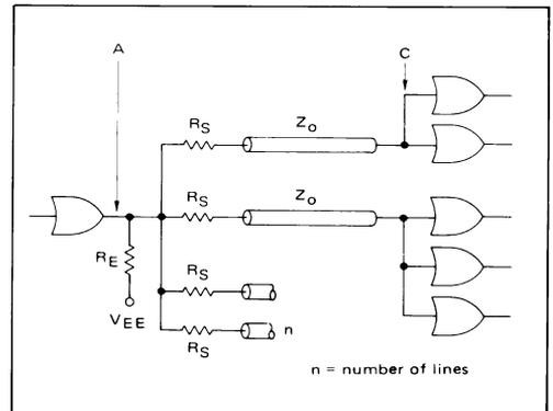
FIGURE 13 — Parallel Fanout with Series Termination
