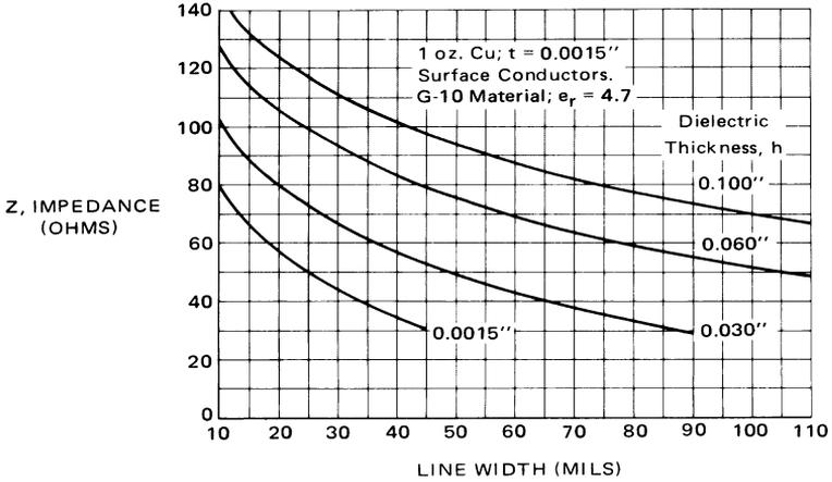
**3-8: Capacitance versus Line Width and Dielectric Thickness for Microstrip Lines**
