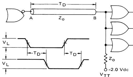
The operation of the parallel terminated line is comparatively simple. The signal swing at point A is:
