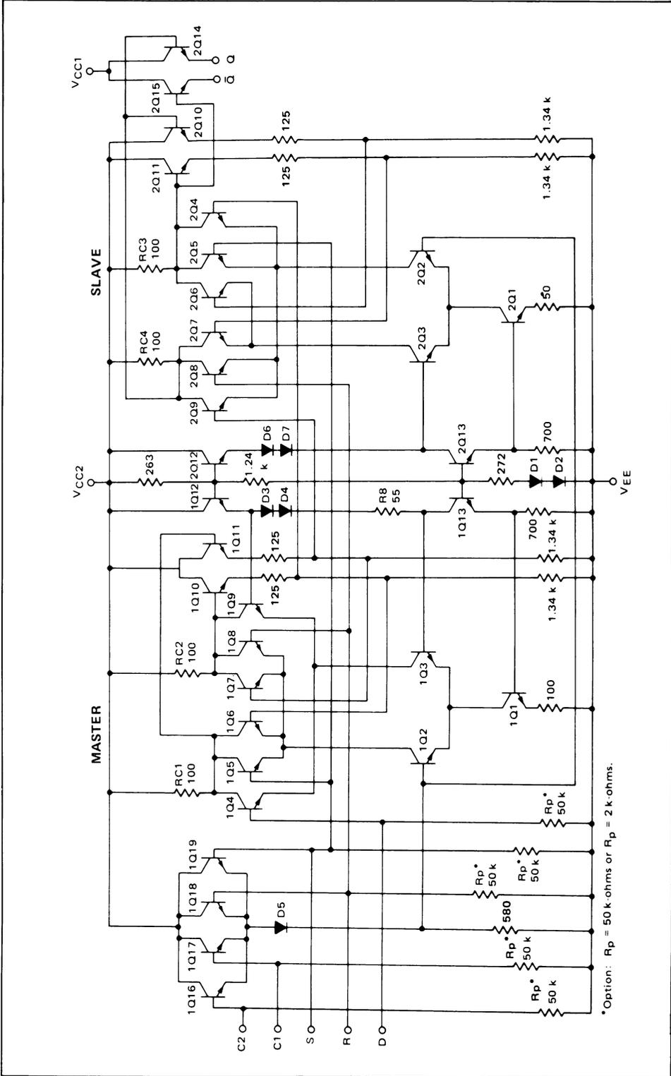
1-8: MECL III Master-Slave Type D Flip-Flop (MC1670)
