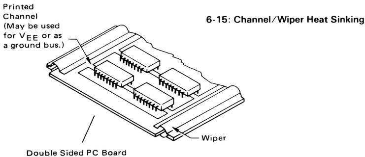
The importance of thermal management cannot be overemphasized. Proper design in this area can result in excellent system performance and increased reliability, especially in MECL III systems where higher power dissipation is encountered.
