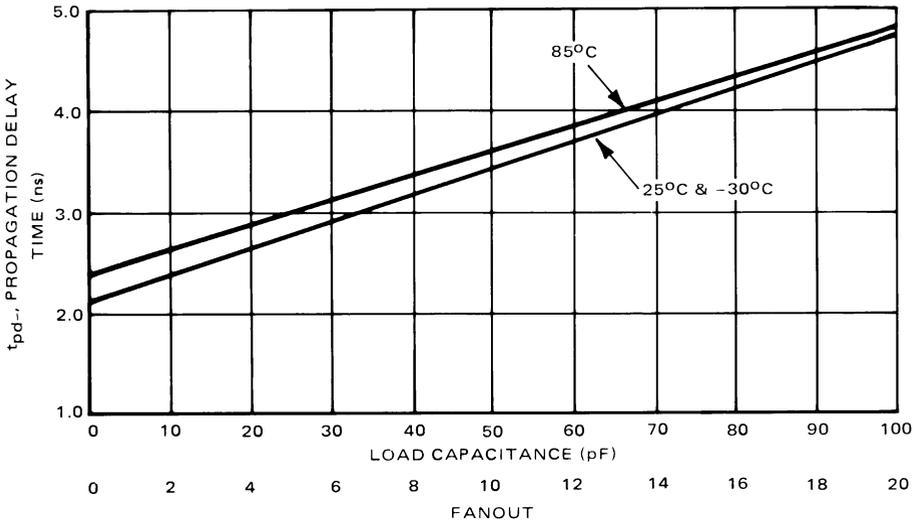
*MECL 10K/10KH Parameters versus Loading and Temperature*
