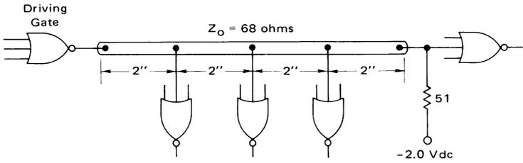
7-22: MECL III Gate Driving a Long Transmission Line with Distributed Loads, and Short Stubs at the Driving Source
