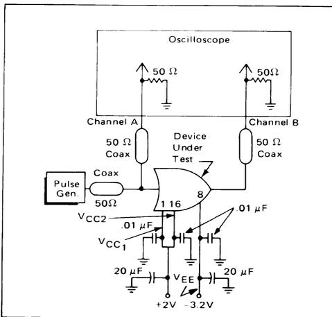
FIGURE 1A - MECL 10K/10KH Test Fixture Schematic
