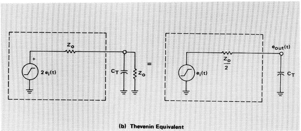
7-24(b). Figure 7-25 shows the Thevenin equivalent for a series terminated line. Note that the impedance ( $Z_0$ ) of the series terminated line is twice as large as that for the parallel terminated line. A general equation can be derived for the output voltage assuming the impedance in the circuit to be R. Then a substitution for R will give the equations for both types of lines.
