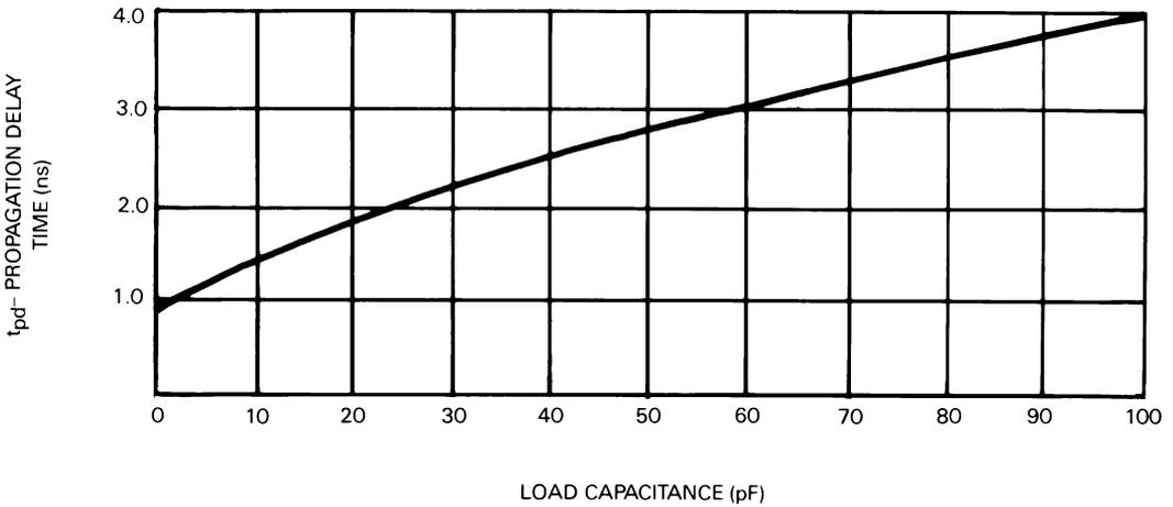
2. Fall-time and  $t_{pd}$  may be improved by using a smaller load resistor between the output and  $-5.2$  Vdc. A  $240 \Omega$  resistor will cut the delay caused by capacitive loading nearly in half. Load resistors less than  $180 \Omega$  should not be used because the heavy load may cause a reduction in noise immunity when the output is in the 1 state, due to increased output emitter-follower  $V_{BE}$  drop. Normally  $510 \Omega$  load resistors provide a good speed-power system design.
