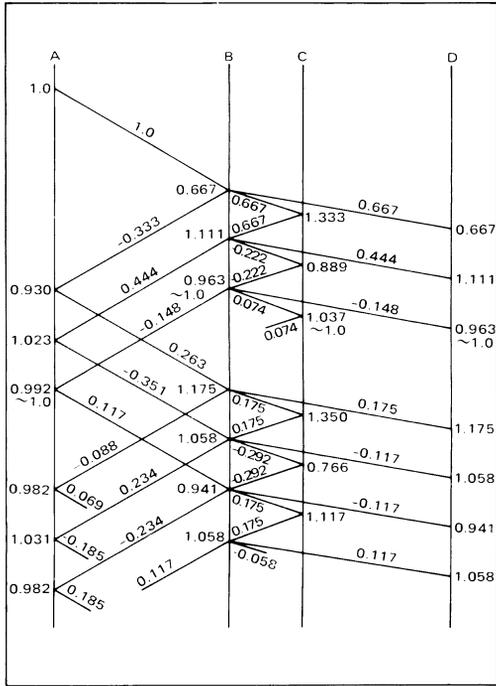
FIGURE 9 — Lattice Diagram for End-Driven Line with Stub
