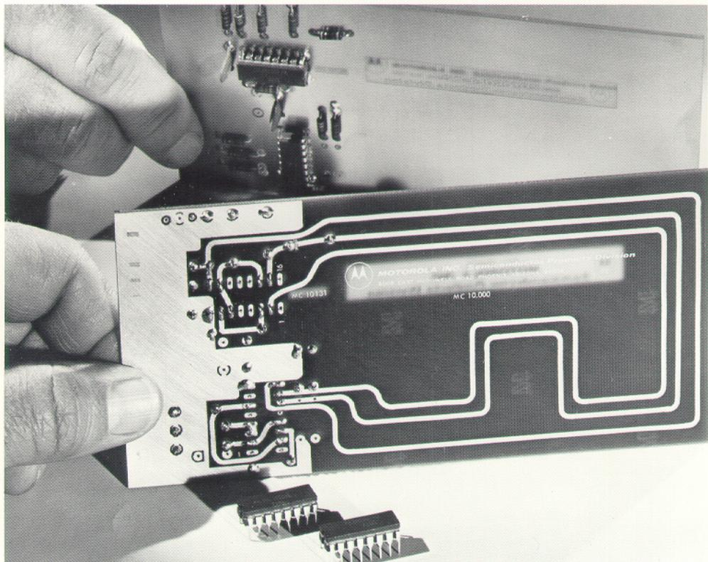
Conventional two-sided printed circuit board can be used when designing with MECL 10K/10KH. Shown is a demonstration board which illustrates some of the capabilities of MECL 10K series parts.
