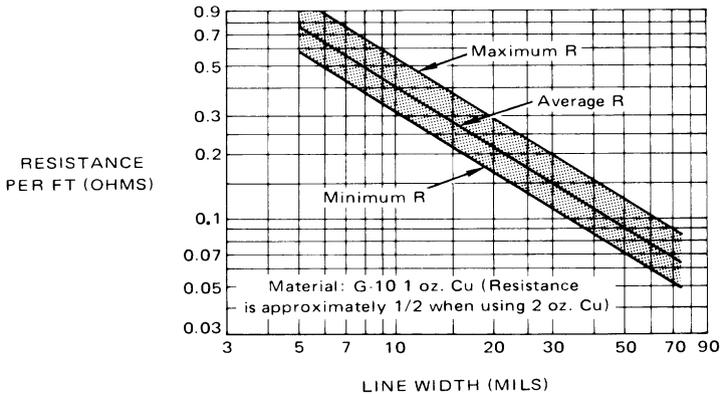
where  $V_{OH}$  is the logic 1 output voltage and  $R_T$  is the terminating resistor. Normally this signal voltage drop is small and need not be calculated. For example, 7 feet of 15-mil wide line will have less than 30 mV drop. The maximum length allowable will be that for which  $\Delta V$  remains below about 100 mV.
