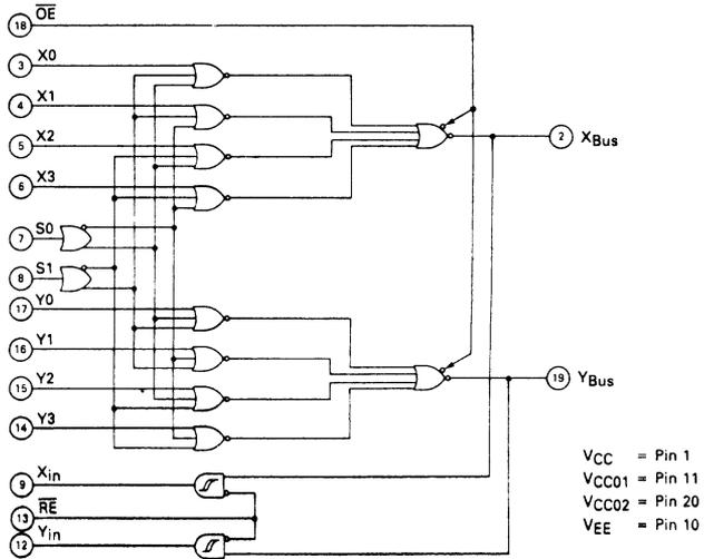
FIGURE 6 — LOGIC DIAGRAM (MC10H332)
