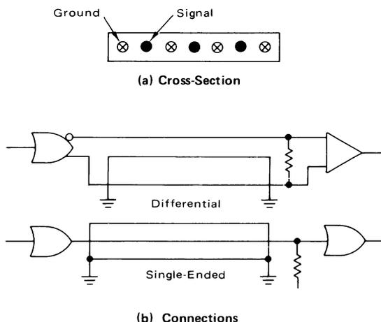
Another type of multiconductor cable is called “triax.” As its name suggests, this is a three-conductor cable with characteristics similar to coaxial cable. Triax has a flat cross section for flexibility, and may be used with all MECL families including MECL III. When using triax type cables, the manufacturer should be consulted for information about the impedance and attenuation characteristics of a specific cable type.
