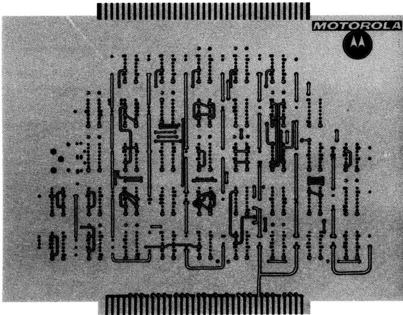
FIGURE 5 – MECL 10,000 PC Board With Ground Plane
