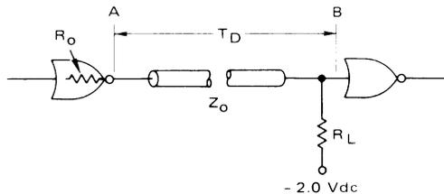
loads at both ends. For the purpose of discussion the line delay will be long with respect to the rise time so that reflections will appear at their full amplitude. The output voltage swing at point A is a function of the internal voltage swing, output impedance, and line impedance:
