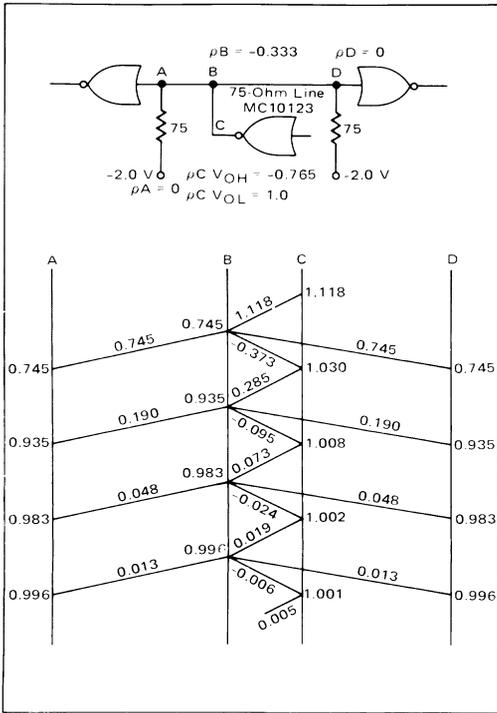
FIGURE 12 — Lattice Diagram for Center-Driven MECL Bus
