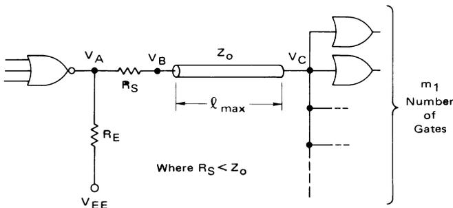
*Output Voltage from a Series Damped Line*
