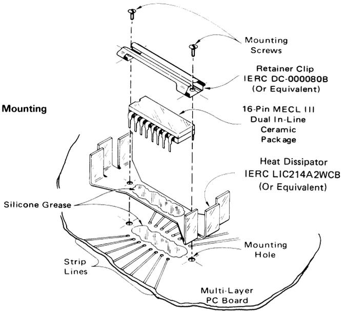
it is possible to use the MECL III counter in still air at  $25^{\circ}\text{C}$  and maintain the die temperatures within rated limits.
