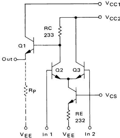
Proceeding with the numerical calculations gives  $g_m = 3.9 \cdot 10^{-2}$ , and voltage gain = 9.0 V/V.
