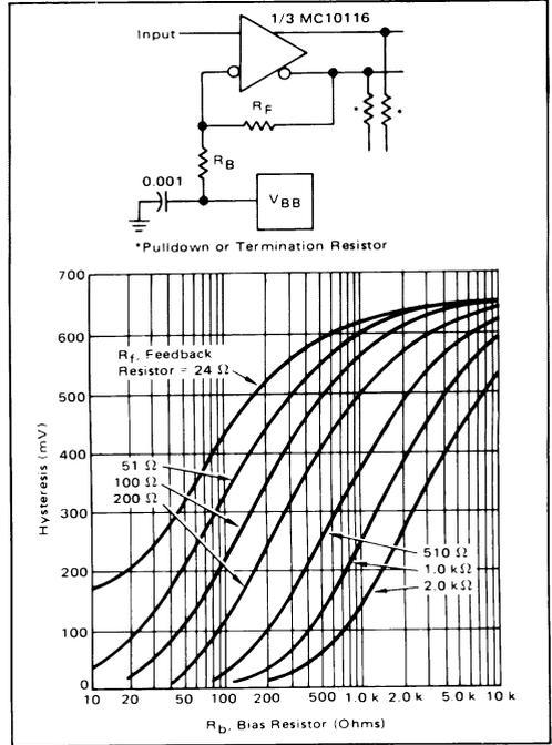
FIGURE 14 – MECL Schmitt Trigger and Hysteresis Curves
