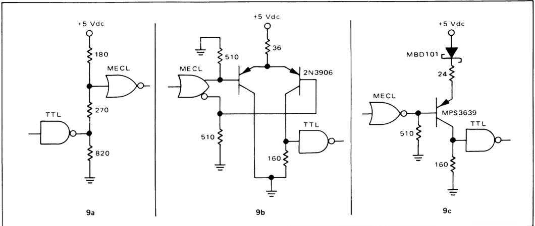
FIGURE 9 — Common Supply ECL/TTL Interface Circuits
