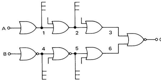
Under heavy loading, propagation delay along path A will be less than along path B because of the use of OR outputs in A as opposed to the NOR outputs in B. This difference (Figure 2-10) is due to the effect of loading on the fall time, rather than being due to a timing difference between OR and NOR outputs. As a matter of fact, under light loading, propagation delays for both NOR and OR outputs are identical.
