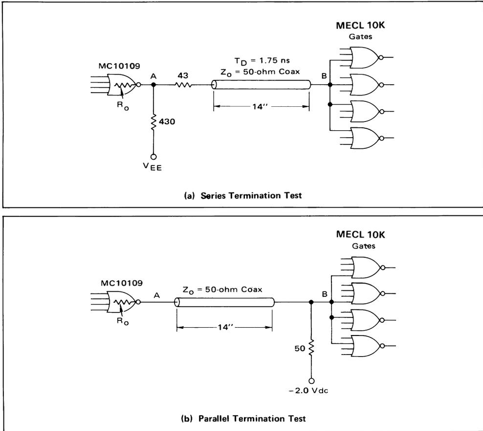
Since the propagation delay increase is twice as much for a series terminated line as for a parallel terminated line, an equation similar to equation 11 can be derived. The propagation delay of a series terminated line can be written as:
