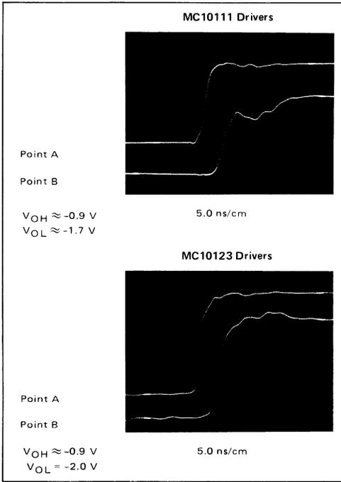
FIGURE 4 — Bus Waveforms at Midpoint
