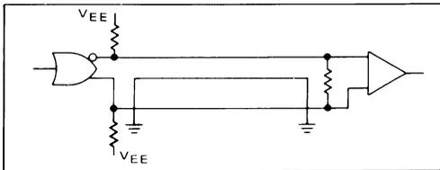
FIGURE 33 – Using Ribbon Cable as Twisted Pair Line
