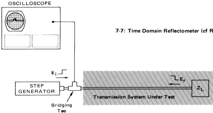
The incident voltage step,  $E_i$ , is a positive edge with an amplitude of 1 volt and a rise time of 30 ps. It is generated by a tunnel diode, which has a source impedance of 50 ohms (HP 1817A sampler, or equivalent). Also, the output edge has very little overshoot (less than  $\pm 5\%$ ).
