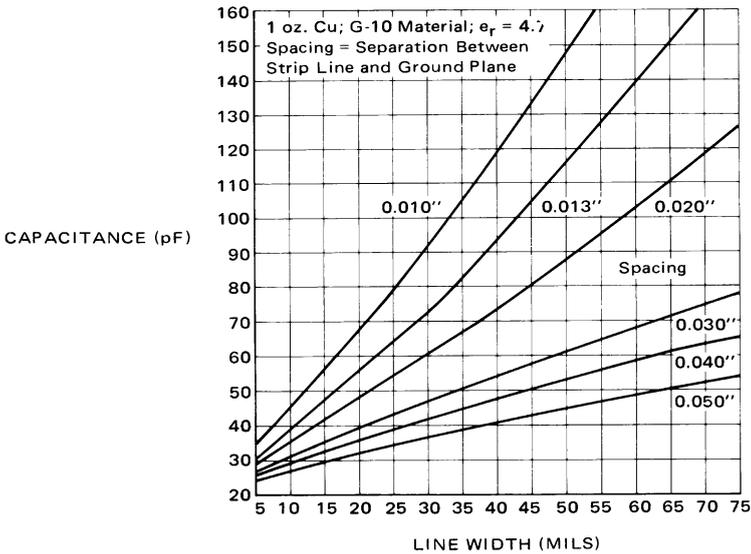
dielectric constant of the medium, and the distance between the ground planes are all controlled, the line will exhibit a characteristic impedance that can be held constant within  $\pm 5\%$ . The characteristic impedance of a strip line is theoretically:
