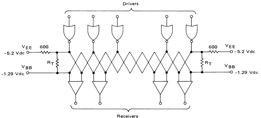
available from the MC10114, MC10115/H115, MC10116/H116, and MC1692L and may be buffered as shown in Figure 4-18 to handle the necessary termination current).
