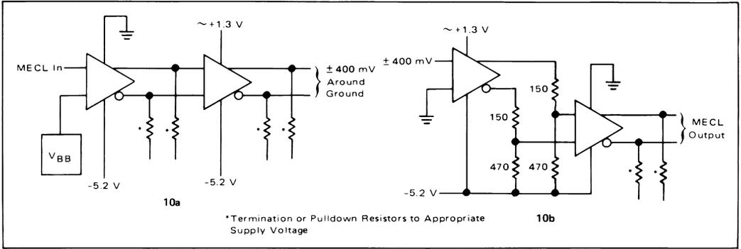
FIGURE 10 – Interfacing with Non-MECL Compatible ECL Using MC10116's
