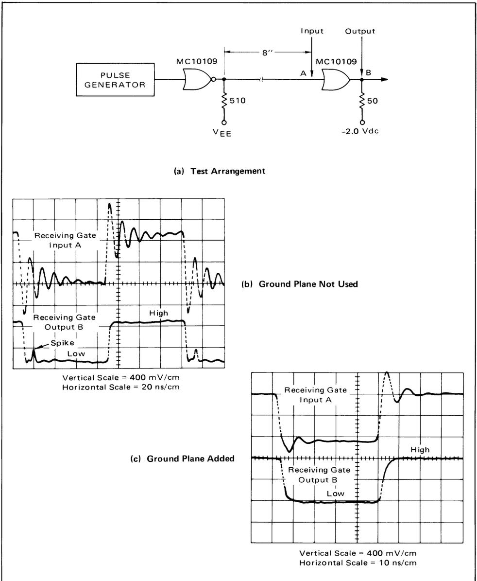
points A and B are shown in Figure 3-1 (b). Trace A shows an overshoot condition of 60% and an undershoot of 40%. It can be seen how this undershoot condition affects trace B during the low level period of the signal — a small spike is produced.
