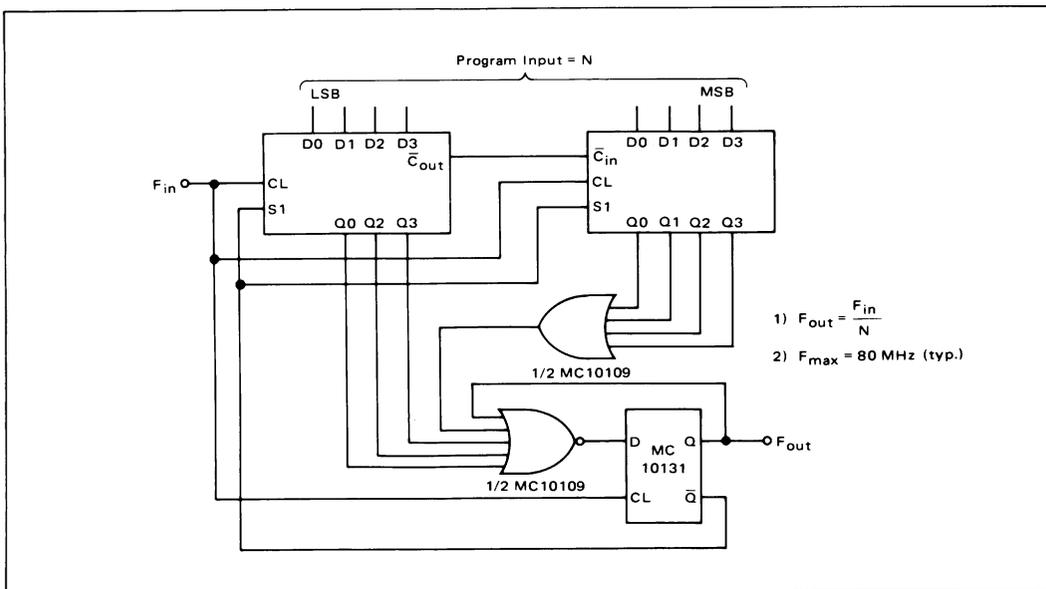
FIGURE 9 – Two-Stage Pulse Gobble Counter. Divide Modulus  $M$  is 255 Maximum with MC10136
