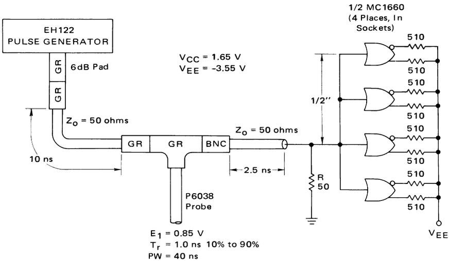
be 275 mV, in a direction indicating it was due to a terminal capacitance,  $C_T$ . A formula may be derived so that the amount of this capacitance can be calculated. Figure 7-19 shows the equivalent circuit which will be used for the derivation of
