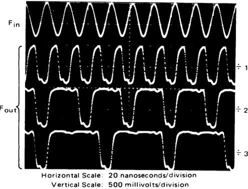
**FIGURE 2 – Programmable Counter Using no External Gating. Divide Modulus M = N + 1.**
