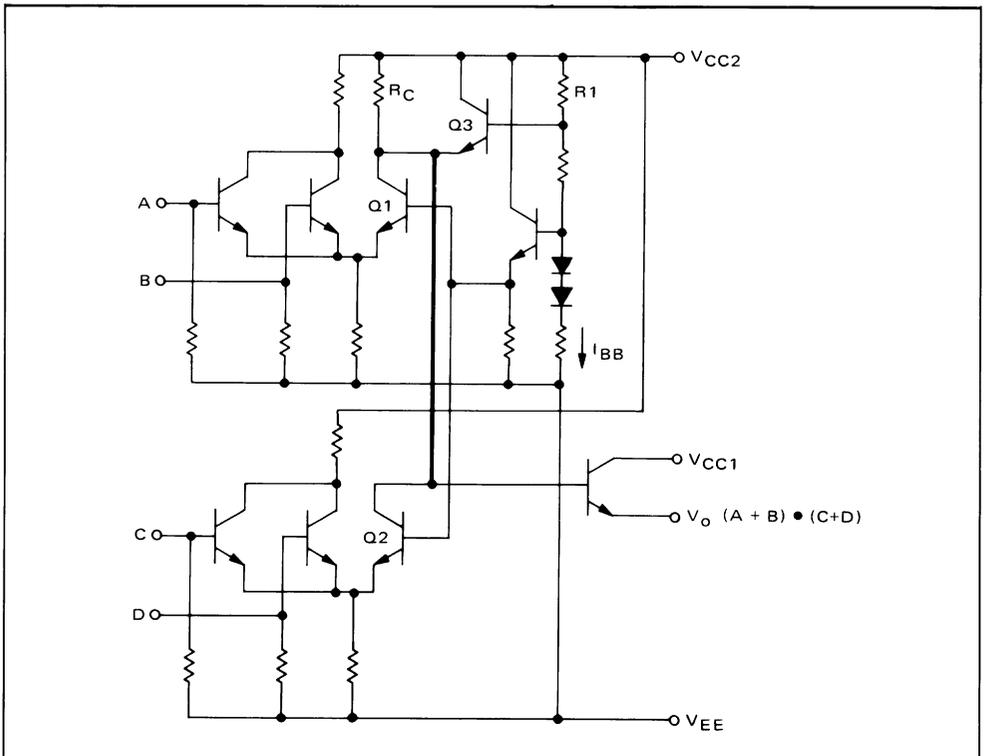
Collector dotting is a second logic technique which is used in the MECL 10K/10KH series. With it, the logic AND function can be generated by interconnecting one collector node of separate differential current switches as shown in Figure 1-7. When connected this way the two 2-input OR gates give the logic function:
