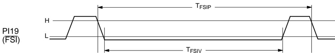
Fig. 12-2: FSI-timing
