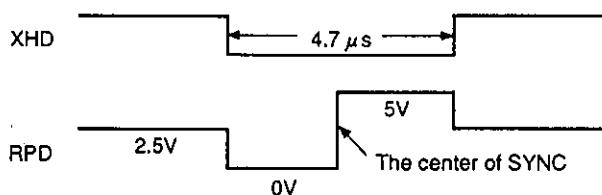
A fully synchronized AFC circuit is built in. PLL error detection signal is generated at the following timing.
