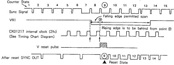
Since the falling edge point in the diagram above (marked with  $\uparrow$  ) is the boundary of reset, if the falling edge of the VRI input traverses that point, it causes 1/2H deviation to the reset state.
