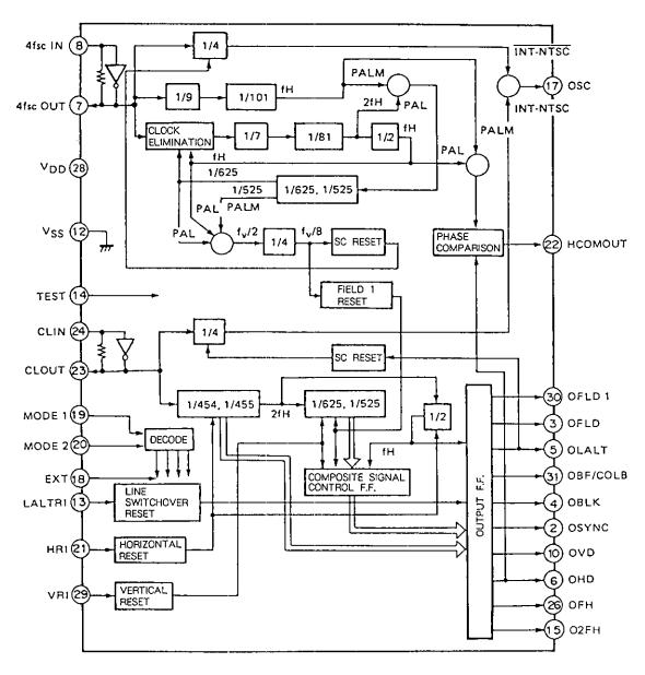
**Note:** Pin 17 output is (a) a signal based on Pin 24 in INT mode at NTSC. (b) each signal is based on Pin 8 in other modes.
