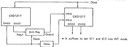
By varying the Delay and Shift Reg. of the above diagram, any phases of OHD2 and OVD2 can be provided against the respective OHD1 OVD1.
