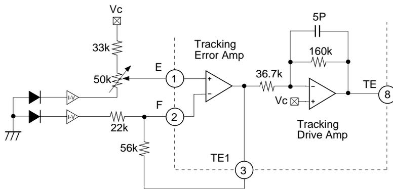
The low frequency gain of TE output voltage is as follows:
