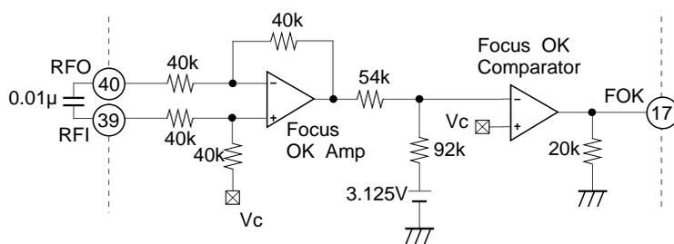
The low frequency component of RF can be gotten by obtaining the difference of the Pins 40 and 39 RF signals, whose low frequency components are removed, at the focus OK amplifier.
