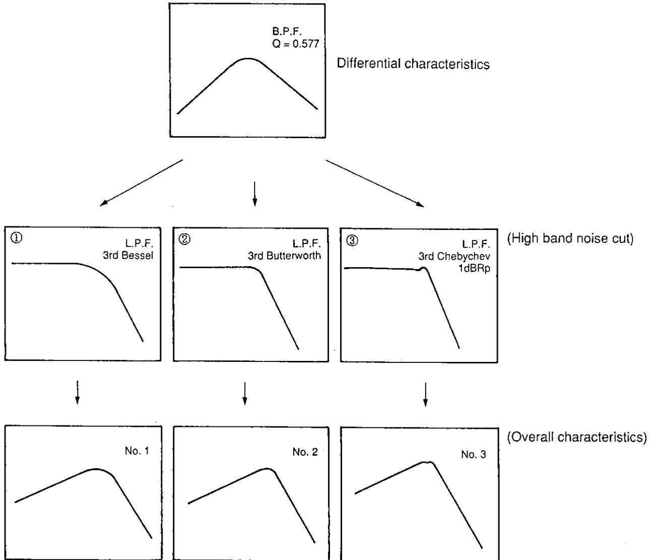
\* No. 1's Bessel characteristics applicable only in 1M/outer track mode.
