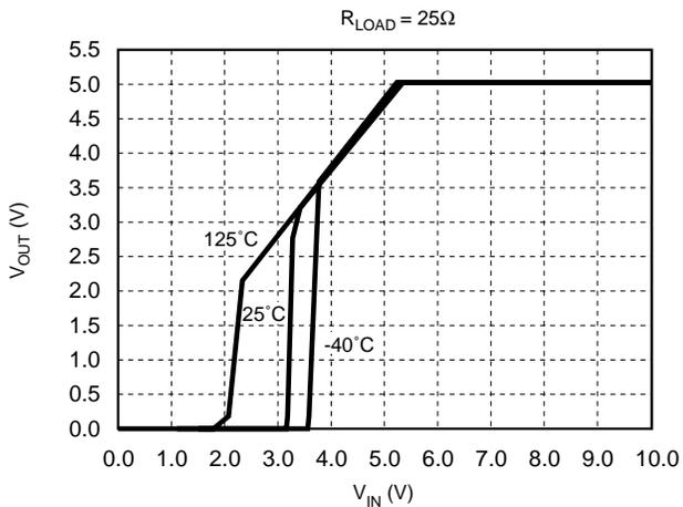
**V<sub>OUT</sub> vs. V<sub>IN</sub> over R<sub>LOAD</sub>**
