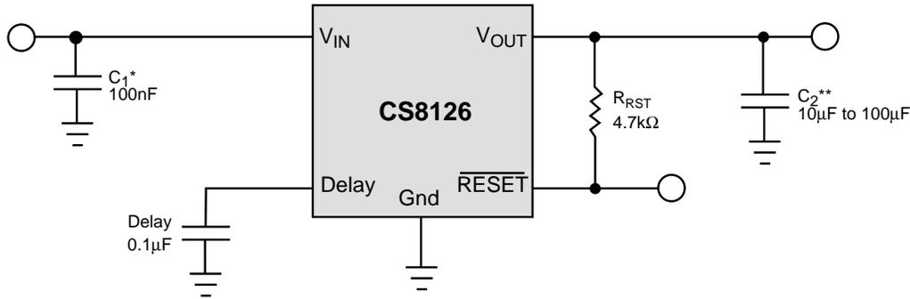
$C_1^*$  is required if the regulator is far from the power source filter.
