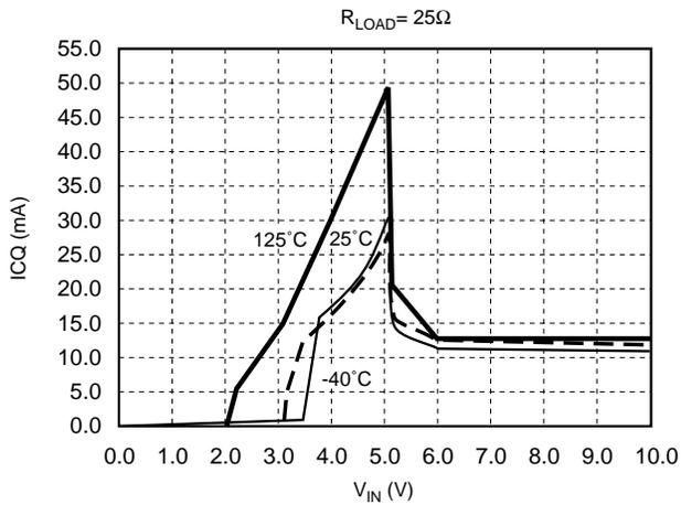
**I<sub>CQ</sub> vs. V<sub>IN</sub> over R<sub>LOAD</sub>**
