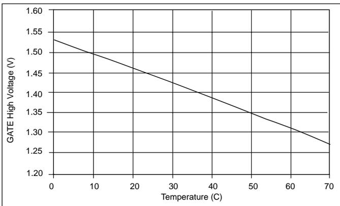
Figure 45: GATE High Voltage (20mA) vs Temperature.
