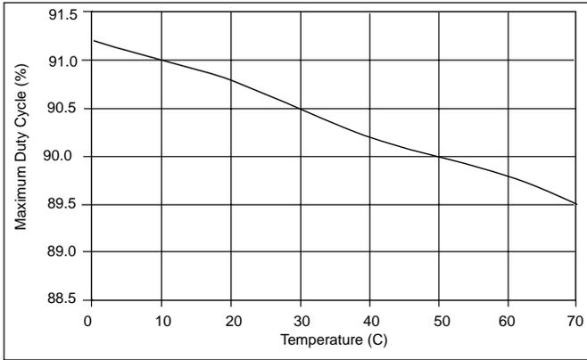
Figure 25: Oscillator Maximum Duty Cycle vs Temperature.
