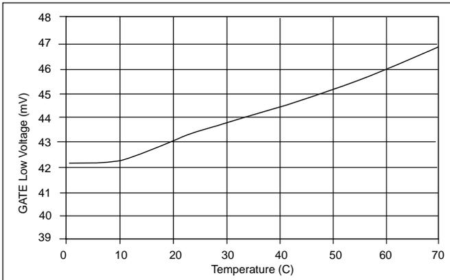
Figure 44: GATE low voltage (20mA) vs Temperature.
