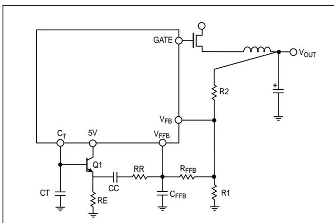
**Figure 4:** Artificial ramp components CC,  $C_{FFB}$ , RR and  $R_{FFB}$  must be provided for each channel if duty cycle for that channel exceeds 50%. Q1 and RE are common to both channels. DC voltage is shown supplied to  $V_{FFB}$  through the  $V_{FB}$  resistor divider.
