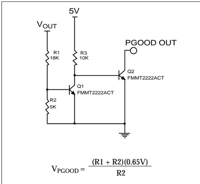
Figure 13: Example external Power GOOD circuit.  $P_{GOOD}(OUT)$  is low until  $V_{OUT}$  exceeds  $V_{PGOOD}$ .  $V_{PGOOD}$  is typically chosen to be 10% below nominal  $V_{OUT}$ . Resistor values above provide a -10% tolerance on  $V_{OUT}=3.3V$ .
