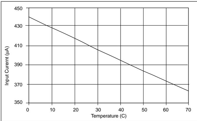
Figure 32: SYNC Input Current vs Temperature ( $V_{SYNC} = 5V$ ).
