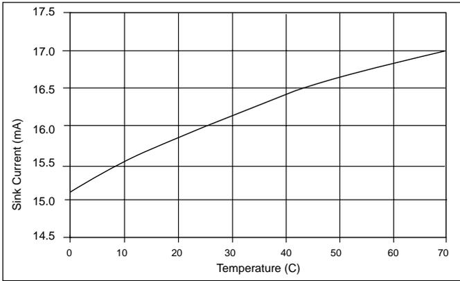
Figure 38: Error Amplifier Sink Current vs Temperature.
