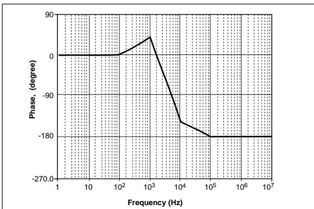
Figure 8: Bode plot of phase response for  $V_{OUT}/V_{CONTROL}$ .
