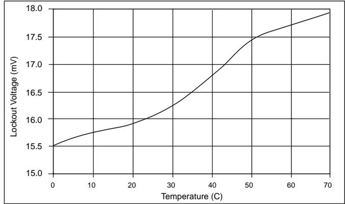
Figure 46: GATE Low Voltage (Lockout) vs Temperature.
