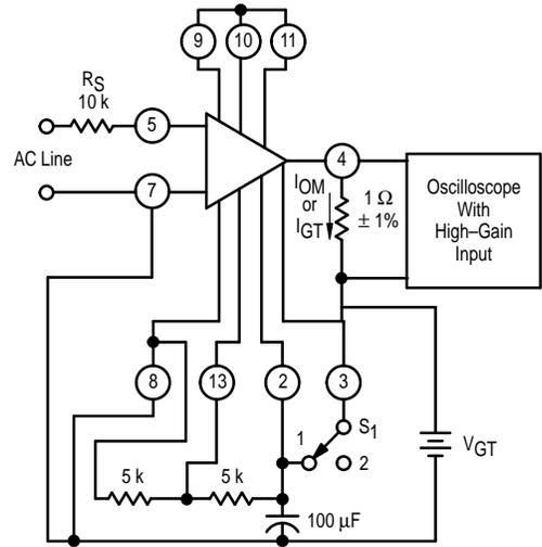
**Figure 4. Peak Output Current (Pulsed) with External Power Supply**
