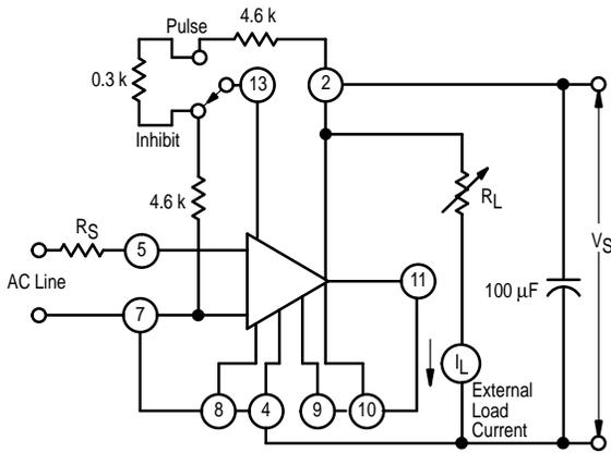
**Figure 3. Peak Output (Pulsed) and Gate Trigger Current with Internal Power Supply**
