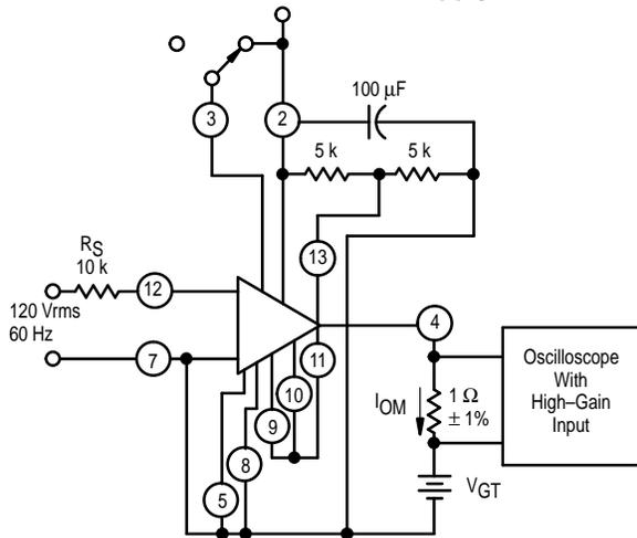
**Figure 5. Input Inhibit Ratio**
