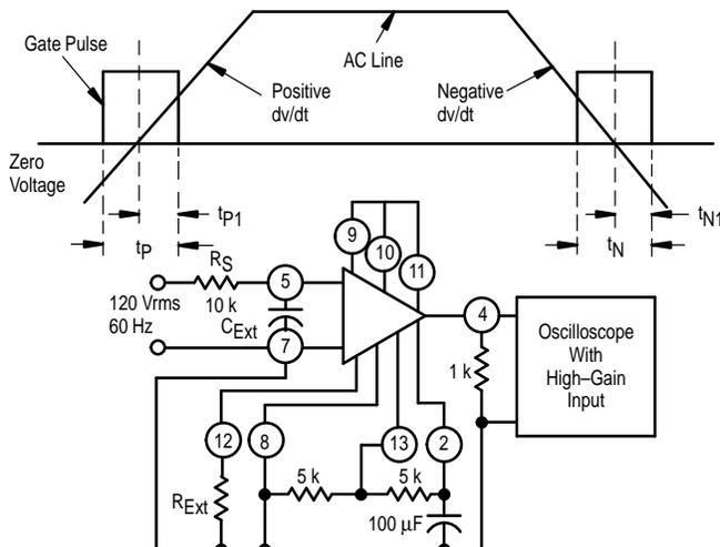
**Figure 7. Input Bias Current Test Circuit**
