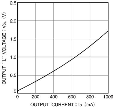
Fig.12 Output low level voltage vs. output current
