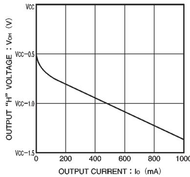
Fig.13 Output high level voltage vs. output current
