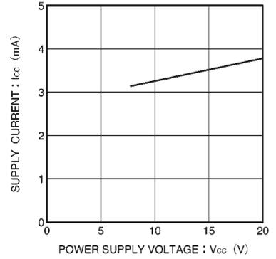
Fig.11 Supply current vs. power supply voltage
