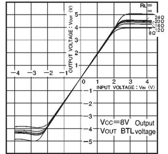
Fig. 5 I/O characteristics (variable load, Vcc = 8V)
