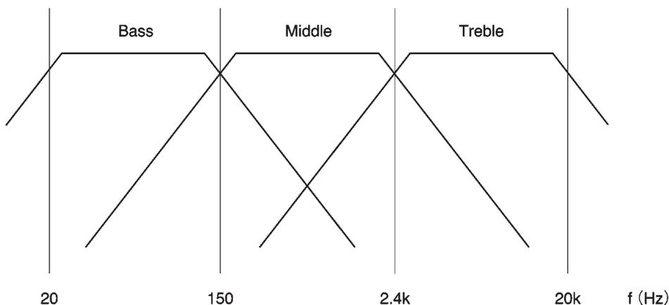
The input signal is separated into three regions : bass (20Hz to 150Hz), middle (150Hz to 2.4kHz) and treble (2.4kHz to 20kHz). These regions are then joined again with the middle and treble regions phase shifted  $-180^\circ$  and  $-360^\circ$  respectively with respect to the bass signal. This phase shift adjusts the delay time characteristic for each band and minimizes the distortion of the rising section of the audio signal.
