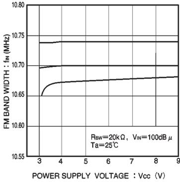
Fig. 5 FM bandwidth vs. power supply voltage
