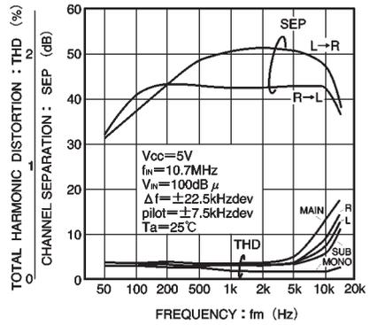
Fig. 6 Channel separation and THD vs. frequency
