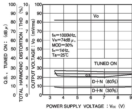
Fig. 8 AM characteristics vs. power supply voltage
