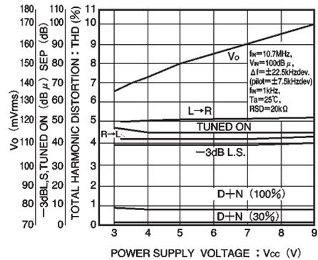
Fig. 4 FM characteristics vs. power supply voltage
