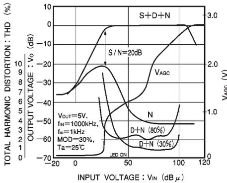
Fig. 7 AM input / output characteristics
