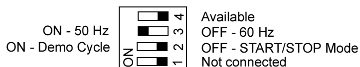
Figure 15. DIP Switch SW1
