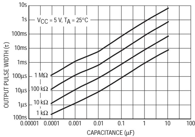
Figure 10. Output Pulse Width vs Timing Capacitance
