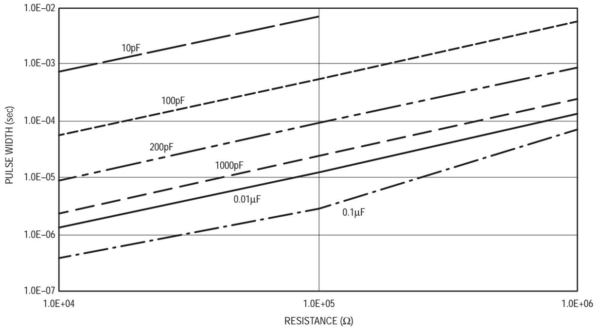
Figure 11. Pulse Width versus Resistance at V<sub>CC</sub> = 3.0V
