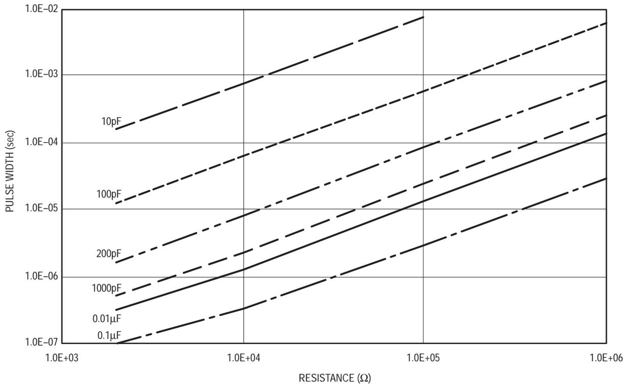
Figure 12. Pulse Width versus Resistance at V<sub>CC</sub> = 4.5V
