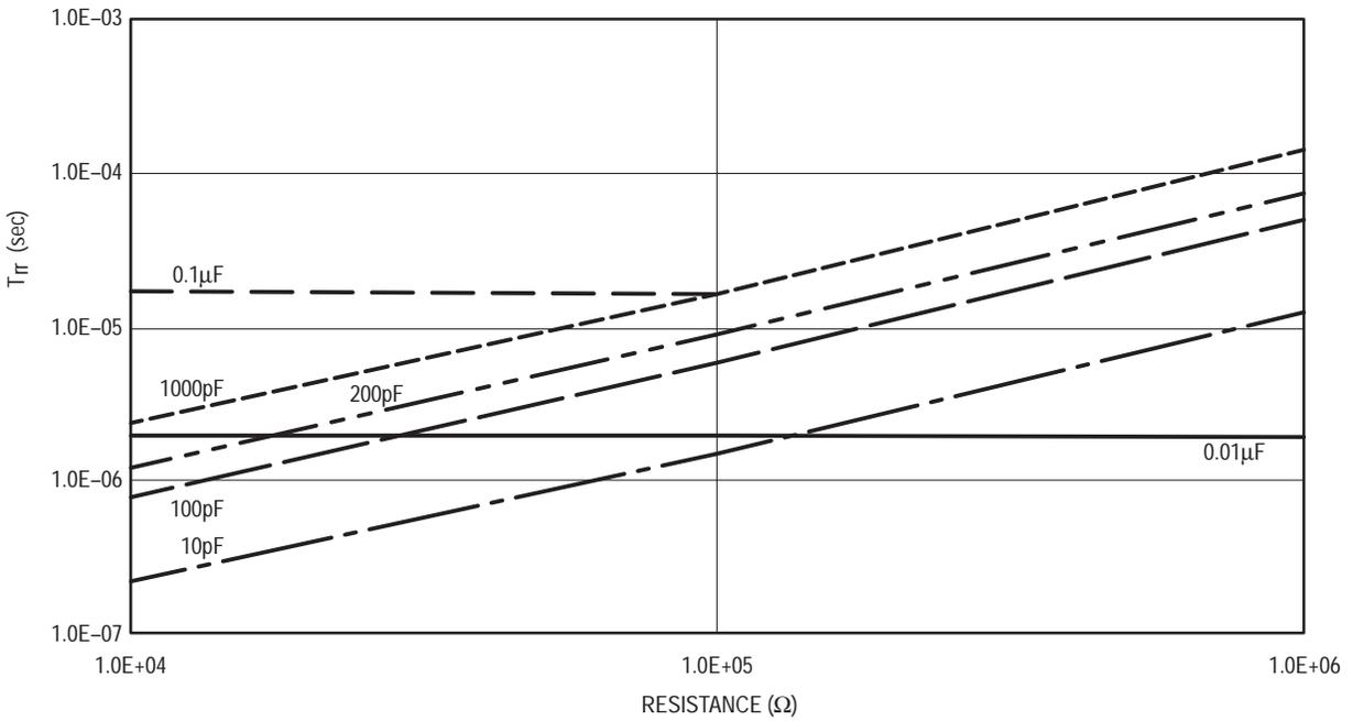
Figure 7. Retrieger Time vs Resistance at  $V_{CC} = 3.0V$
