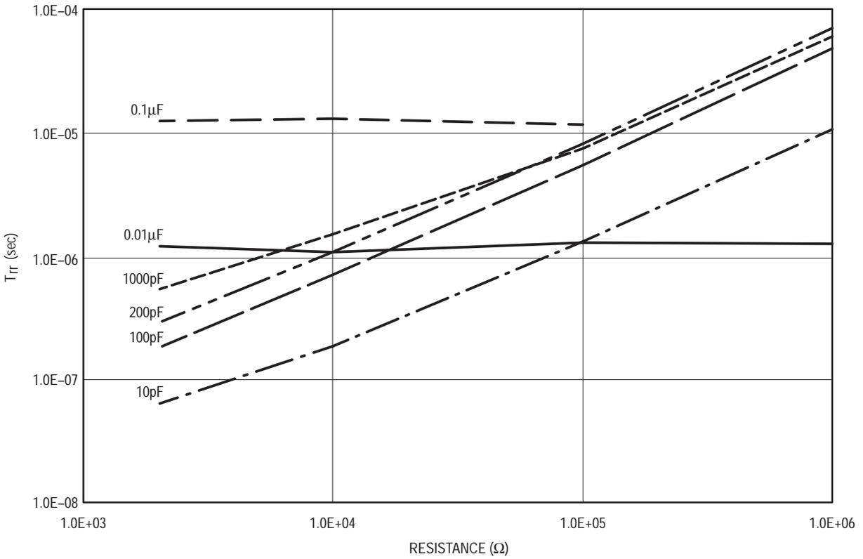
Figure 6. Retrieger Time vs Resistance at  $V_{CC} = 4.5V$
